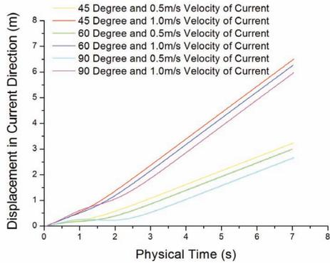
Fig 8 Displacement in Current Direction for Different Ocean Current Velocities and Initial Inclined Angles
