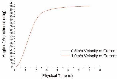
Fig 7 Adjustment of a node in Initial Inclined Angle of 90 Degree
