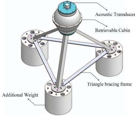
Fig 1 The Structure of UWSN node [8]
