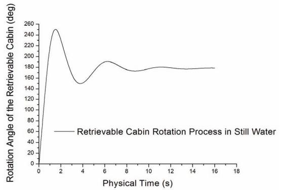
Fig 9 The Recovery Process of Rotation for the Retrievable Cabin
