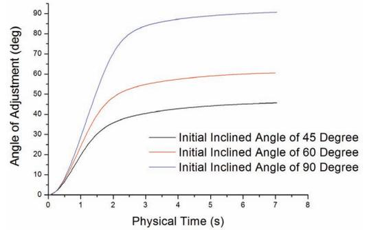
Fig 3 Adjustment of a node in 0.5m/s Ocean Current
