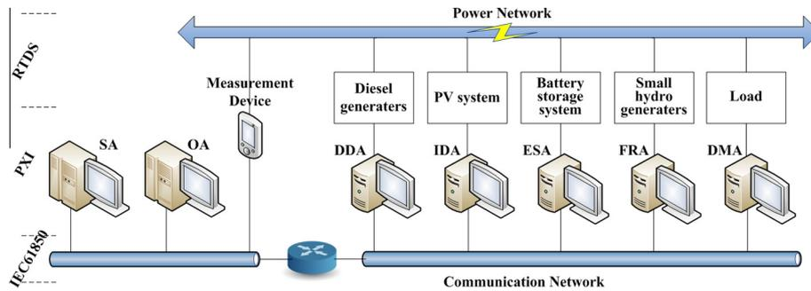
Fig. 7. Implementation of the real-time PXI-RTDS simulation platform.
