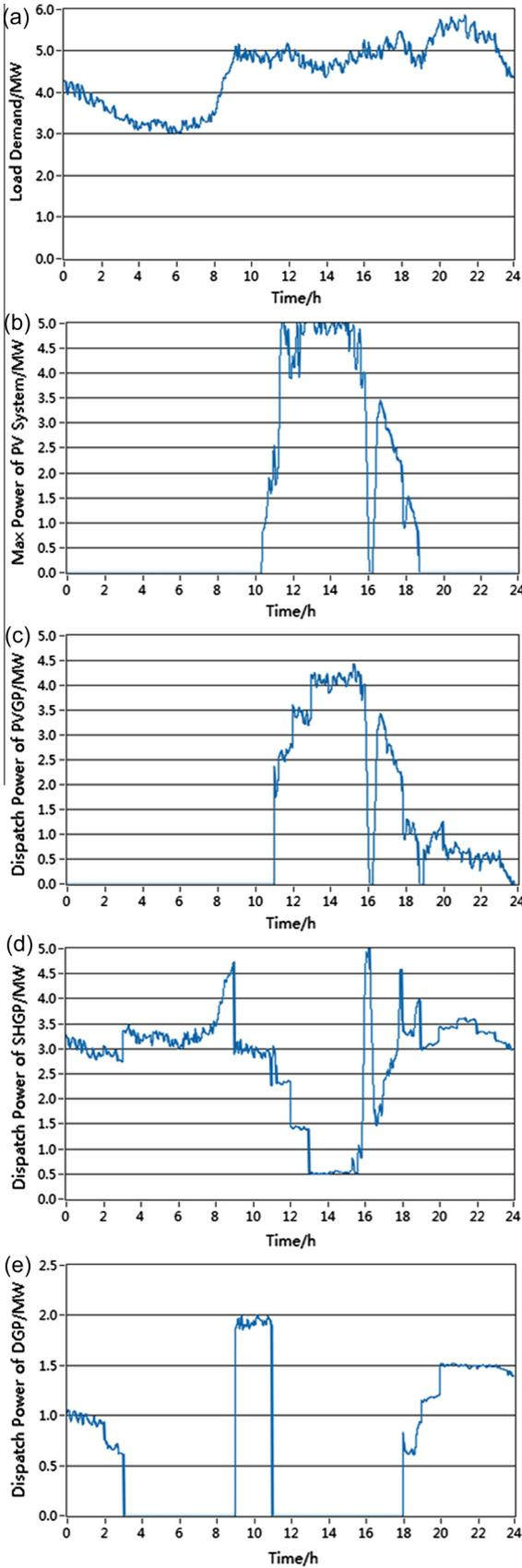
**Fig. 9.** Operation schedule after the dynamic power dispatch: (a) real-time load demand profile, (b) the maximum power that the PV can generate, (c) operation schedule of the PVGP, (d) operation schedule of the SHGP, and (e) operation schedule of the DGP.
