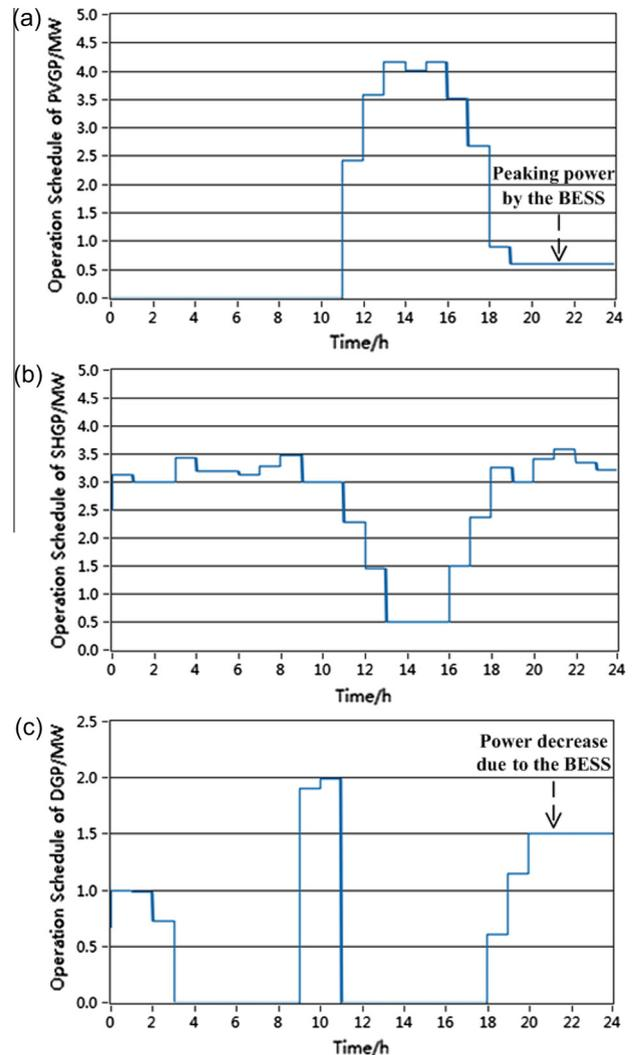
**Fig. 8.** Operation schedule after the VBD: (a) operation schedule of the PVGP, (b) operation schedule of the SHGP, and (c) operation schedule of the DGP.
