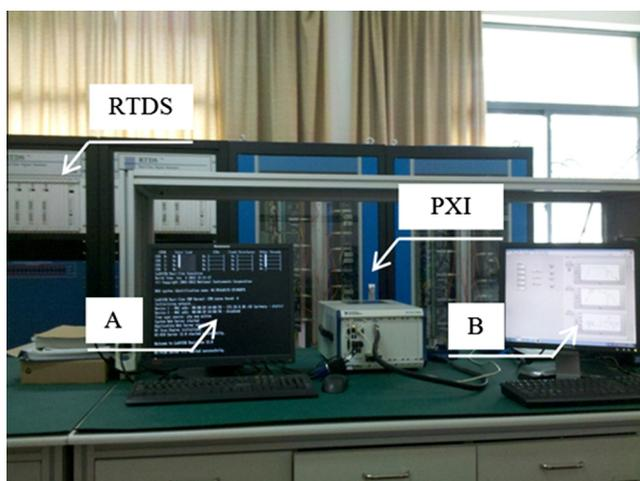
Fig. 5. Photo of the RTDS–PXI real-time simulation platform (A: real-time monitoring of PXI; B: real-time simulation results of MG).
