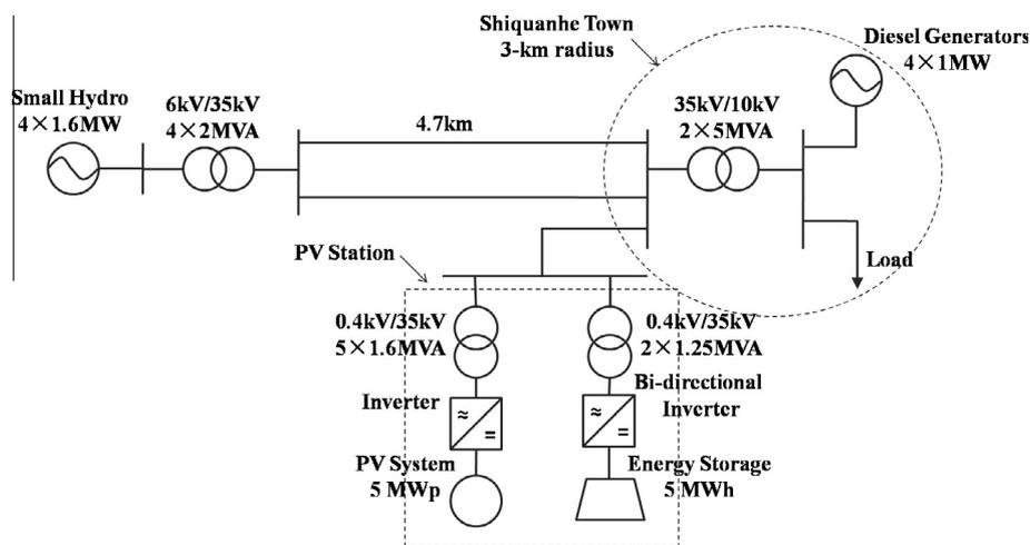
Fig. 1. Configuration diagram of the proposed PVSHH microgrid system.
