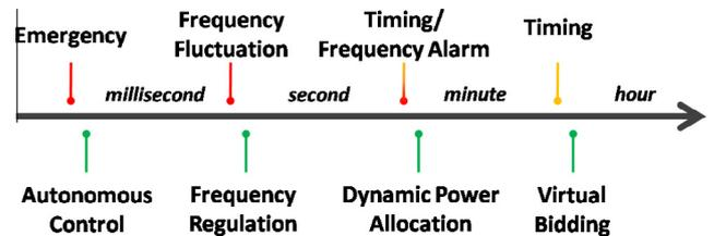
Fig. 4. Dynamic response process of the proposed EMS in different time-scale.
