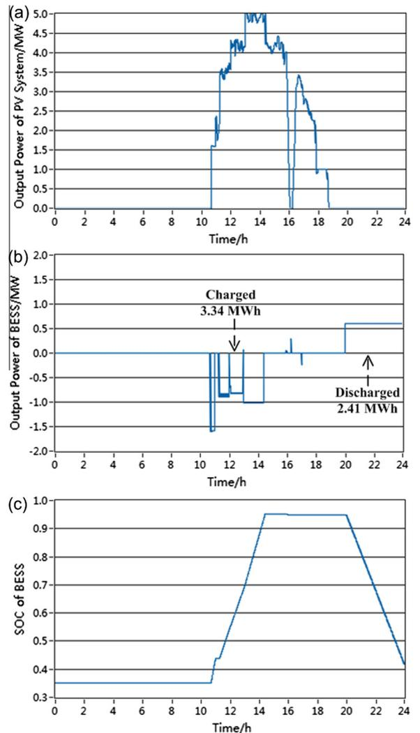
**Fig. 11.** Real-time operation of the PV plant: (a) power generation of the PV system; (b) power generation of the BESS and (c) the SOC of the BESS.
