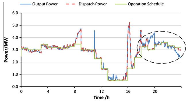
**Fig. 10.** Comparison between operation schedule, dynamic dispatch and actual output of the small-hydro generation plant.
