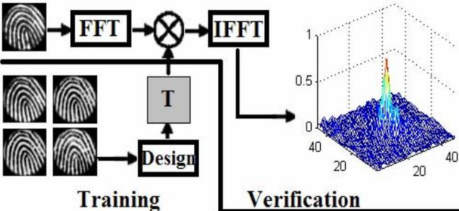
Fig. 3. MACE filter working flow chart on the same sub-type SP correlation.
