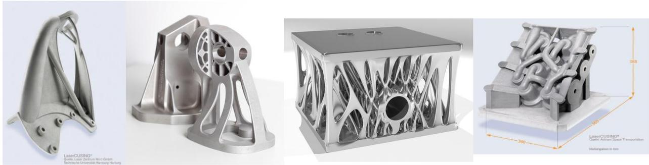
Figure 5 Examples of AM product shapes (courtesy of EOS, Renishaw, Concept Laser)
