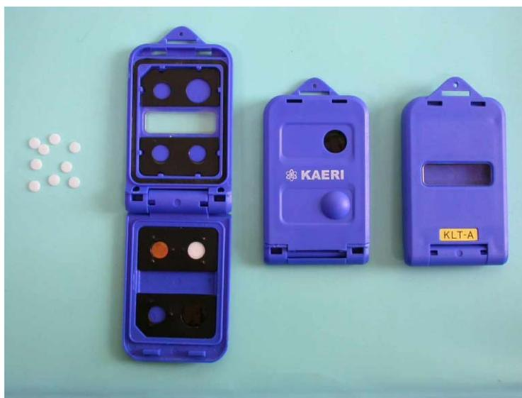
Fig. 5. Photograph of  $\text{LiF:Mg,Cu,Na,Si}$  detectors and the newly developed dosimeter.
