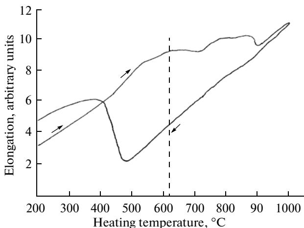
**Fig. 1.** Dilatogram of a vicalloy with 7% V upon heating to 1000°C and cooling (dashed line demonstrates the annealing temperature for producing a high-coercive state).
