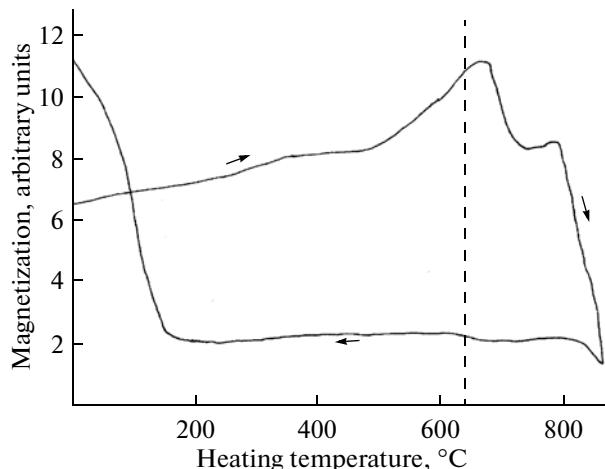
**Fig. 2.** Variation of the magnetization of vicalloy during heating and cooling in the temperature range from 20 to 860°C (dashed line demonstrates the annealing temperature for producing a high-coercive state).
