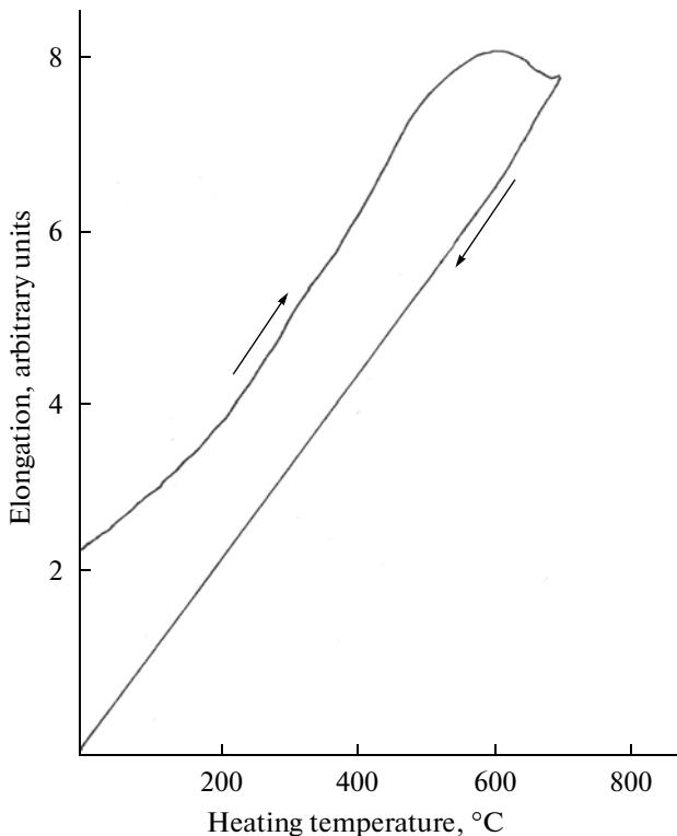
Fig. 3. Dilatogram of the vicalloy upon heating to 690°C and cooling.
