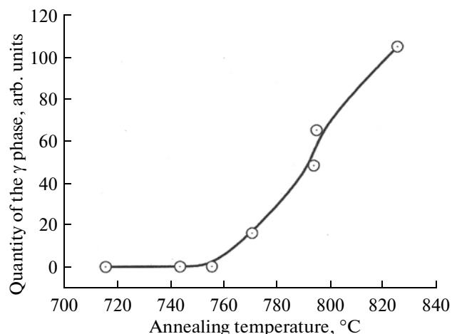
Fig. 4. The amount of the  $\gamma$  phase upon heating of the vicalloy as a function of the annealing temperature.
