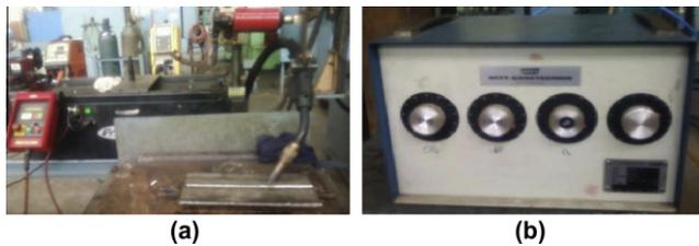
**Fig. 2.** Welding setup (a – carriage, and b – gas mixer).
