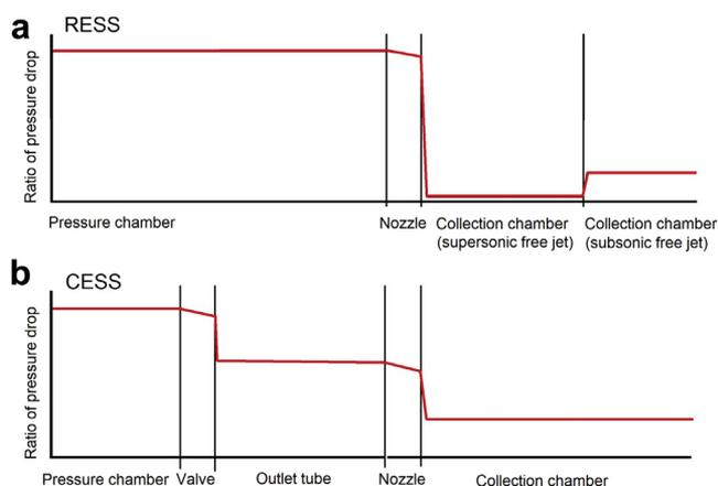
**Figure 2.** Schematic picture describing RESS and RESS process. Pressure within (a) the RESS and (b) the CESS system. Pressure drop in RESS modified from the study by Martin and Cocero.<sup>34</sup>
