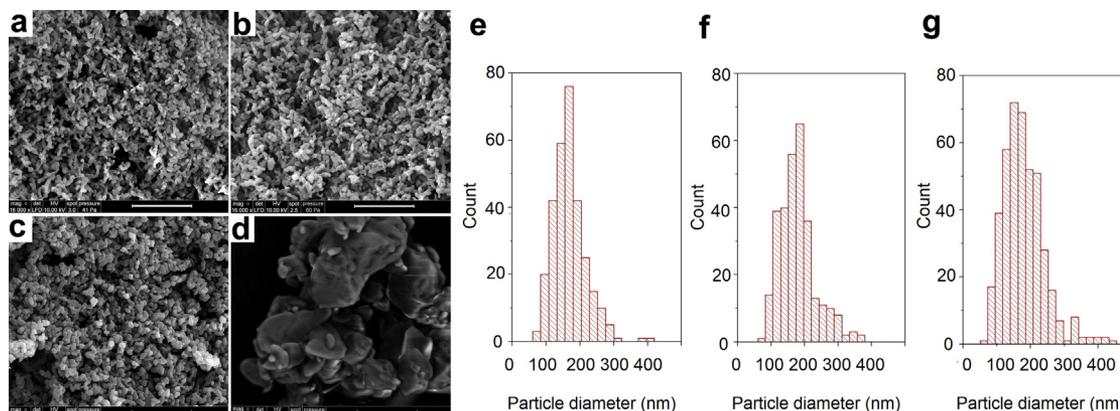
**Figure 3.** Nanoparticles and bulk piroxicam: (a) batch 1, (b) batch 2, (c) batch 3, and (d) bulk piroxicam. The size bar is 5  $\mu\text{m}$ . Particle size distributions with mean particle size and standard deviations for (e) batch 1, (f) batch 2, and (g) batch 3.
