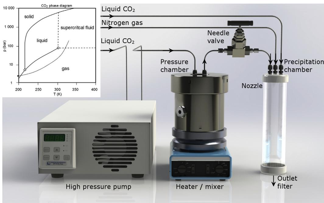
**Figure 1.** Experimental apparatus used to produce nanoparticles. Inset shows the thermodynamics of CESS.
