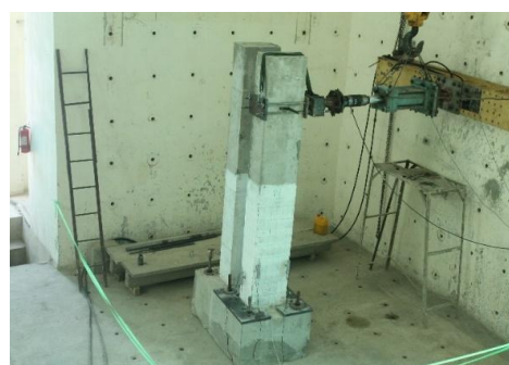
Figure 3: Specimen Construction & Setup, adopted from Ahmad et al. (2016)
