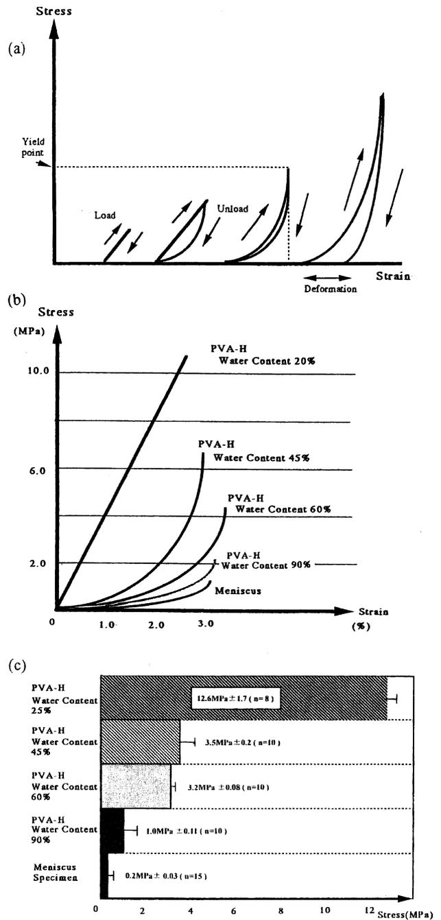
Fig. 3. (a) Measurement of yield point in stress–strain curves of this compression test. (b) Typical stress–strain curves of PVA-H samples and natural meniscus specimens (compression test). (c) Comparison of the yield stress of PVA-H and meniscus specimens.
