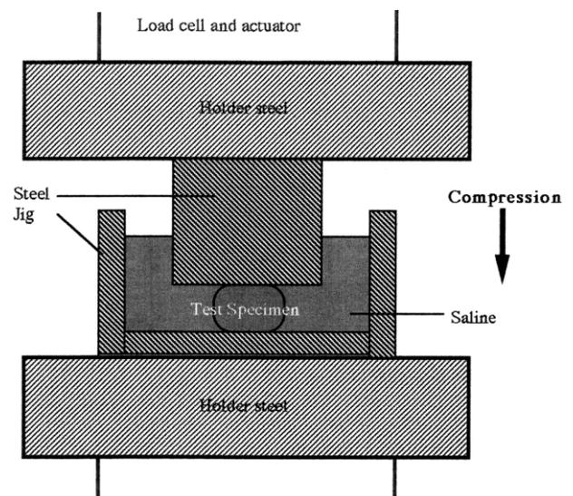
Fig. 2. Diagram of the apparatus for mechanical testing in saline. In this test, the steel holder-transmitted load cell of the autography machine moved at  $5 \text{ mm/min}$  and the stress and strain values of PVA-H and meniscus specimens were measured.
