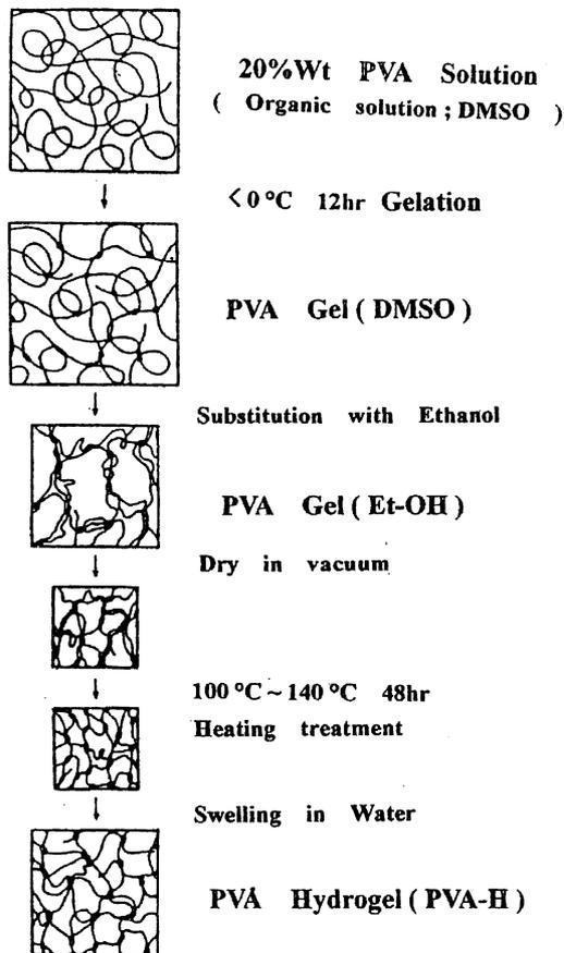
Fig. 1. The manufacturing process of PVA-H.
