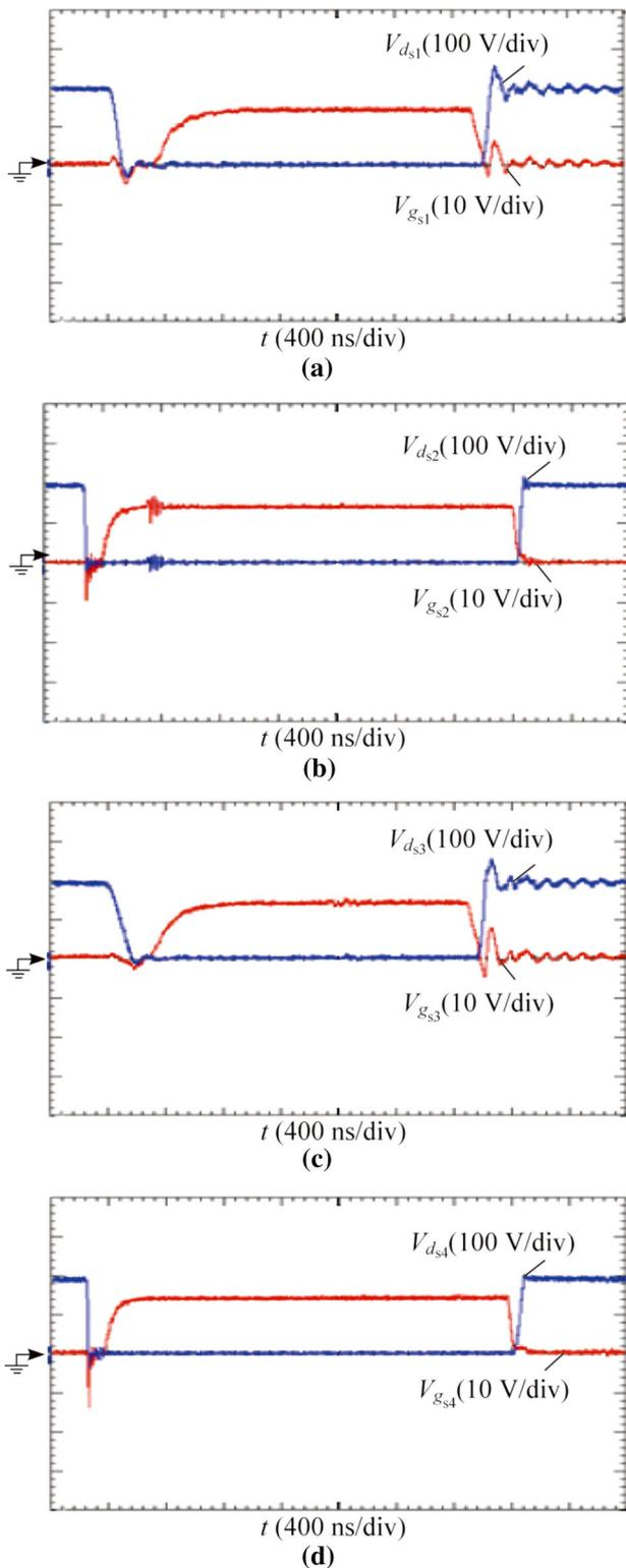
Fig. 8 ZVS soft switching performance in buck mode
