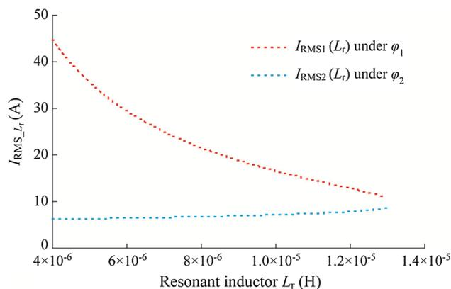
Fig. 5 RMS currents of resonant inductor  $L_r$  under  $\varphi_1$  and  $\varphi_2$  ( $P = 1$  kW)
