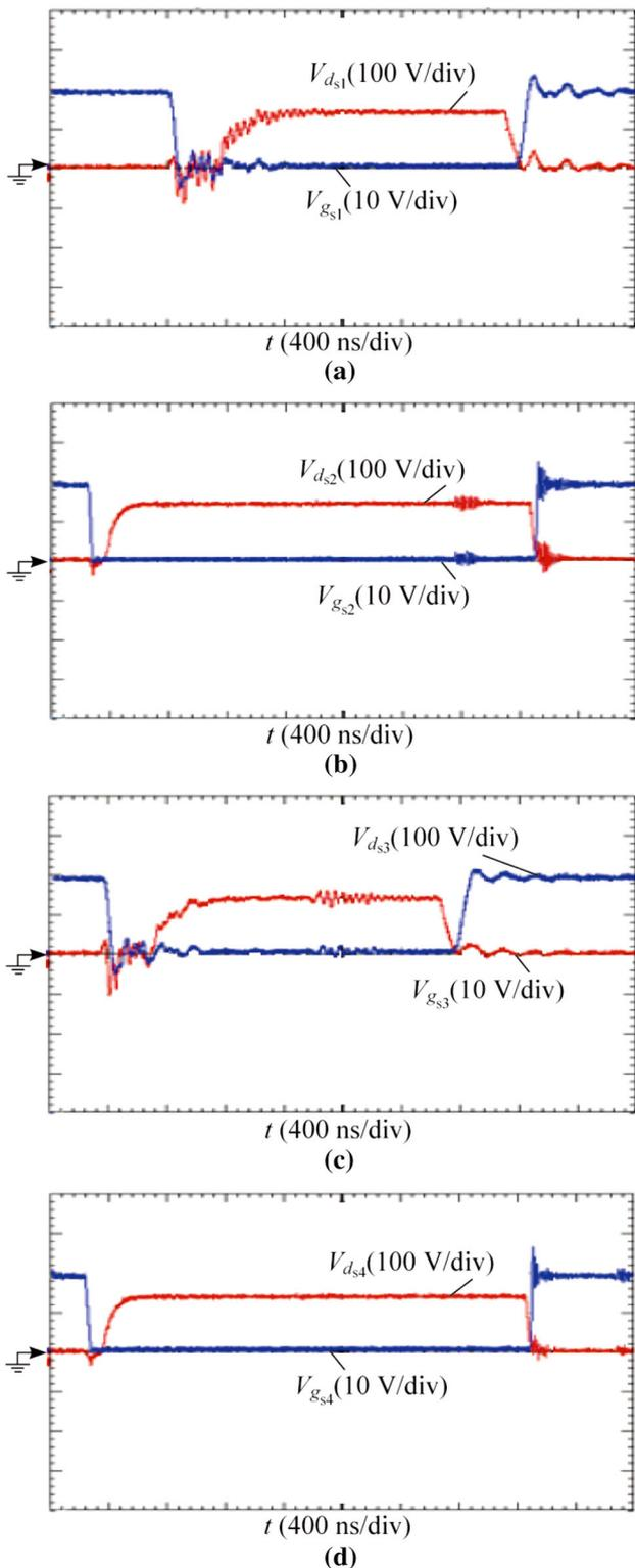
Fig. 10 ZVS soft switching performance in boost mode
