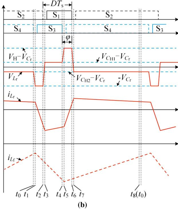
Fig. 2 Steady-state waveforms of stacked converter
