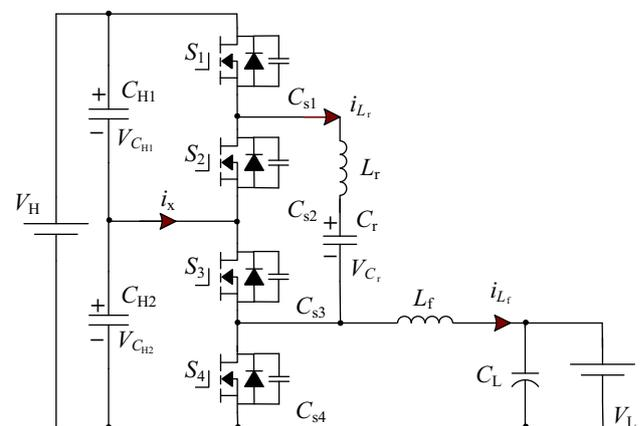
Fig. 1 Stacked bidirectional converter
