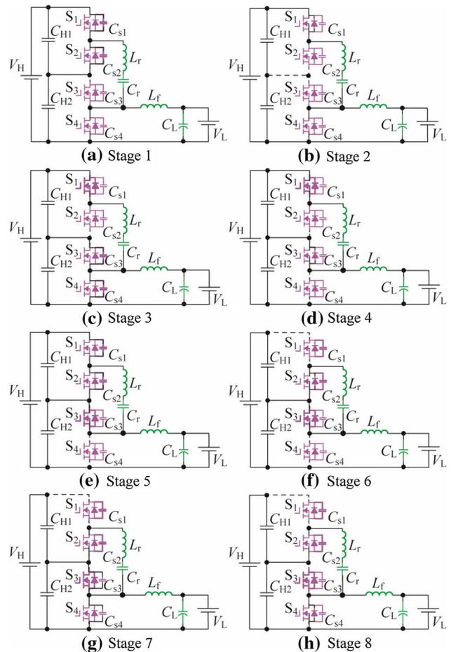
Fig. 3 Equivalent operation circuits of introduced converter
