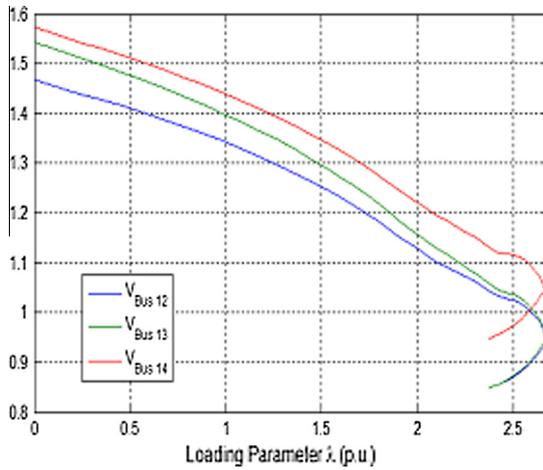
Fig. 10. PV curves after placement of UPFC's.
