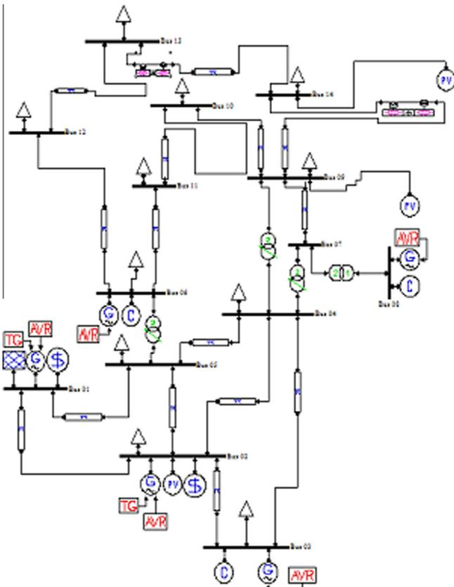
**Fig. 6.** 14-Bus system with UPFC's placed in the optimal location (for line 16 outage).
