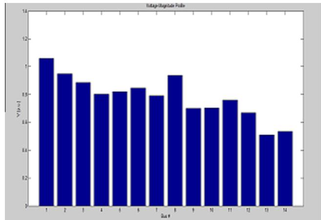
**Fig. 7.** Voltage magnitude profile before placement of UPFC's.
