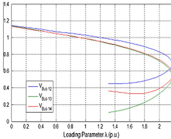
Fig. 9. PV curves before placement of UPFC's.
