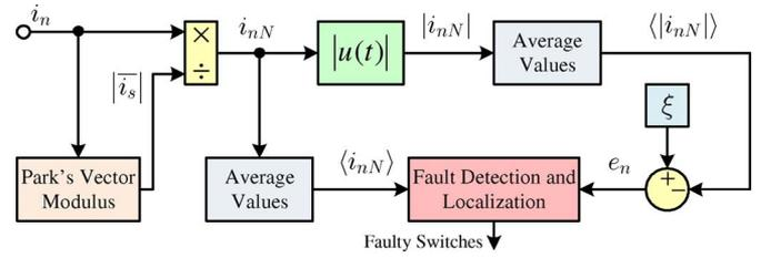
Fig. 1. Block diagram of the proposed fault diagnostic method.
