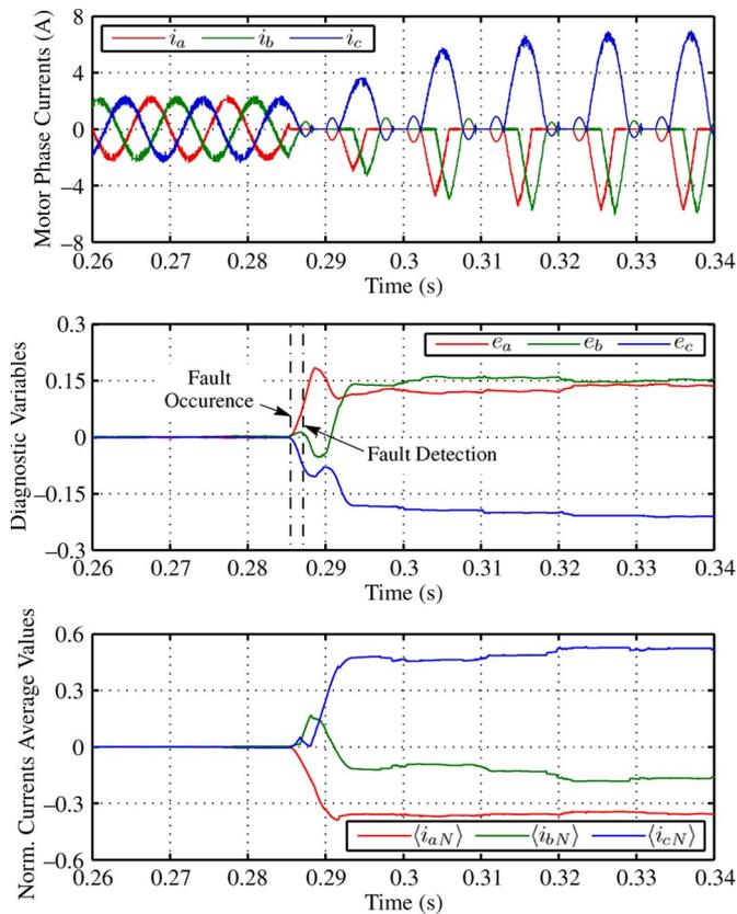
Fig. 10. Experimental results concerning the time-domain waveforms of the motor phase currents, the diagnostic variables, and the normalized currents' average values, for a double power switch open-circuit fault in IGBTs T1 and T3.
