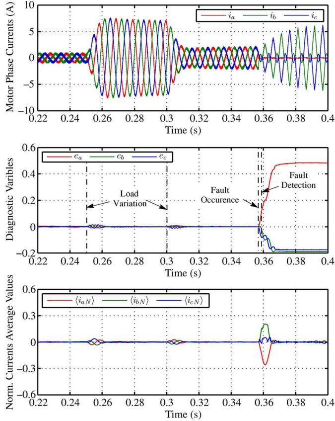
Fig. 4. Simulation results concerning the time-domain waveforms of the motor phase currents, the diagnostic variables, and the normalized currents average values, for a single-phase open-circuit fault in phase  $a$ .
