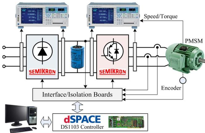
Fig. 8. Block diagram with the components of the experimental setup.
