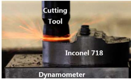
Fig. 9. Measurement of the cutting forces.
