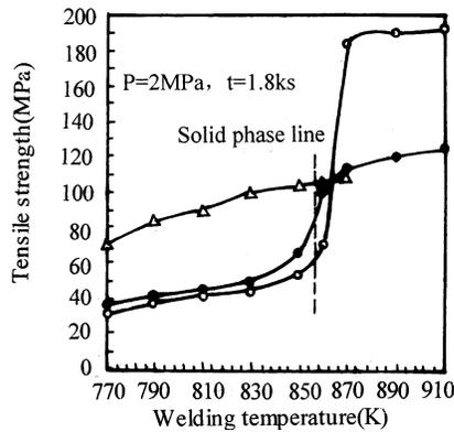
Fig. 3. Relationship between temperature and tensile strength of welded joint □, 6061Al–6061Al, ●, MMC–6061Al, ○, MMC–MMC.
