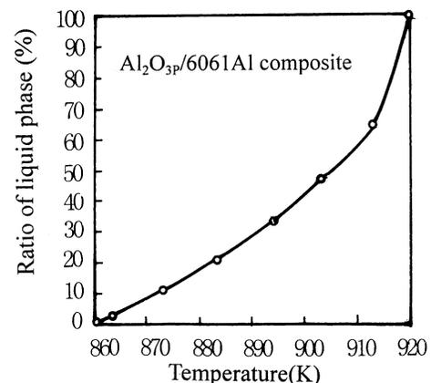
Fig. 2. Volume fraction of the liquid phase matrix as a function of temperature.
