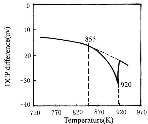
Fig. 1. Determination of the liquid-solid co-existing range of  $\text{Al}_2\text{O}_3/6061\text{Al}$  composite by differential scanning calorimetry.
