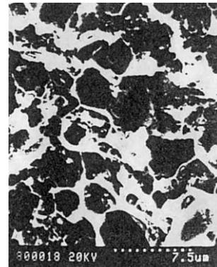
Fig. 6. Fracture surface of aluminium matrix composite  $\text{Al}_2\text{O}_3/\text{6061Al}$ .
