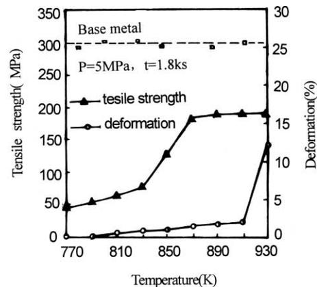
Fig. 7. Relationship between temperature and tensile strength of welded joint.
