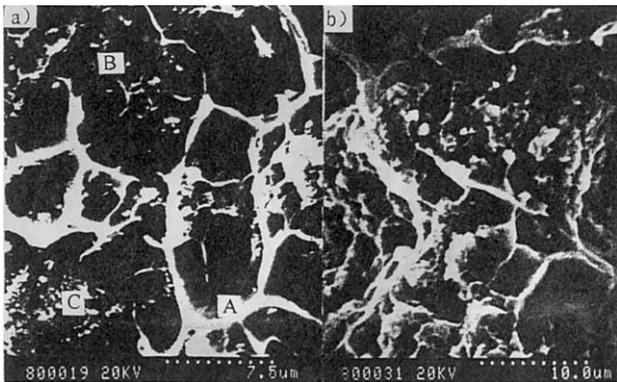
Fig. 4. Effect welding temperature on fractograph of MMC–6061Al, (a) 850 K, (b) 860 K.
