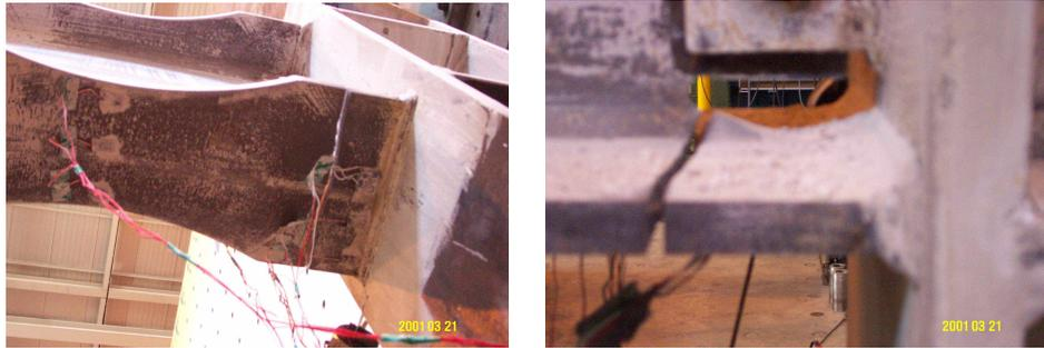
**Fig.6 Beam bottom flange fracture of specimen DB700-SB at 2% story drift**
