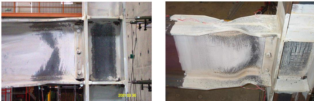
**Fig. 7 Connection region of specimens DB700-MW and DB700-SW**
