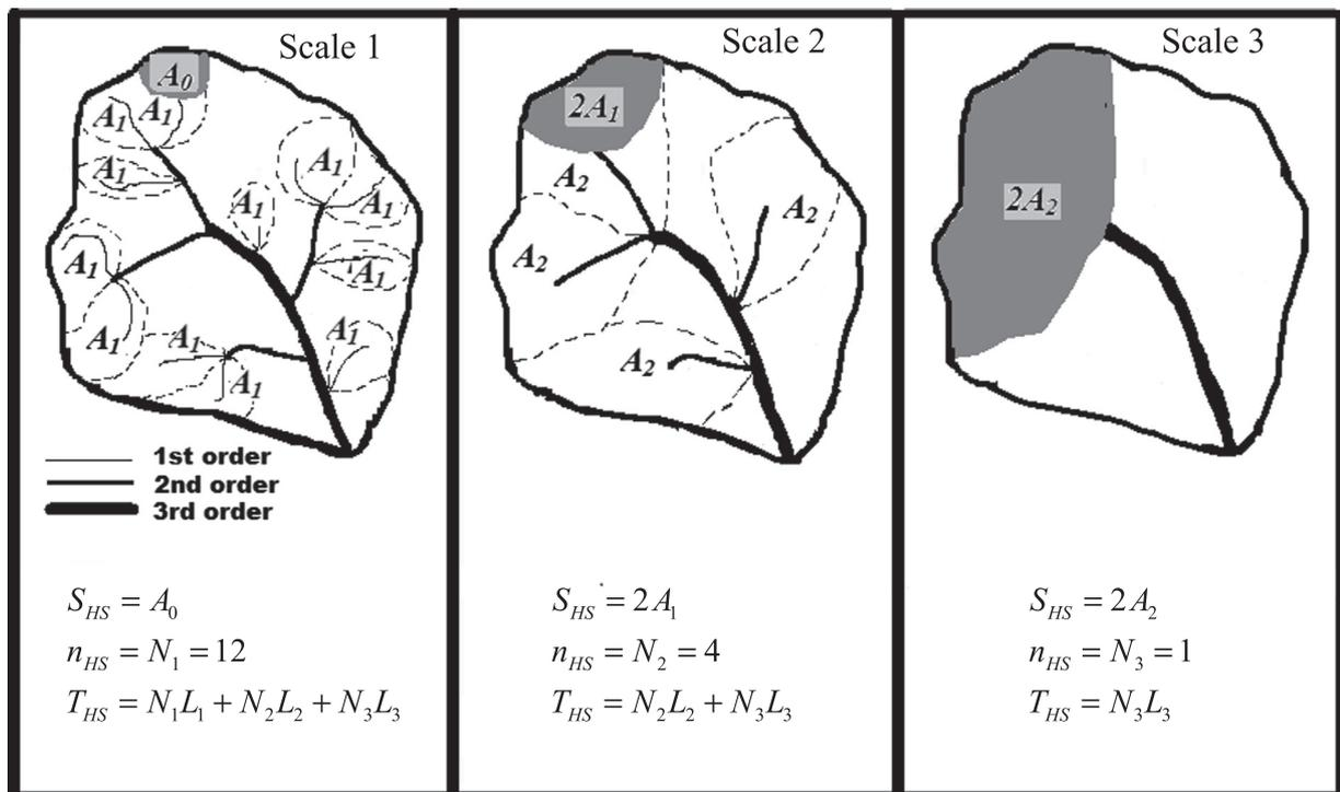
Fig. 1. Stream network demarcated in a catchment corresponding to three different Horton–Strahler scales of observation defined in terms of threshold area  $S_{HS}$  (in km<sup>2</sup>). Analogous figure can be found in Moussa (2009, Fig. 11).  $n_{HS}$  (dimensionless value) denotes number of sources, and  $T_{HS}$  is total length of channel network (in km).
