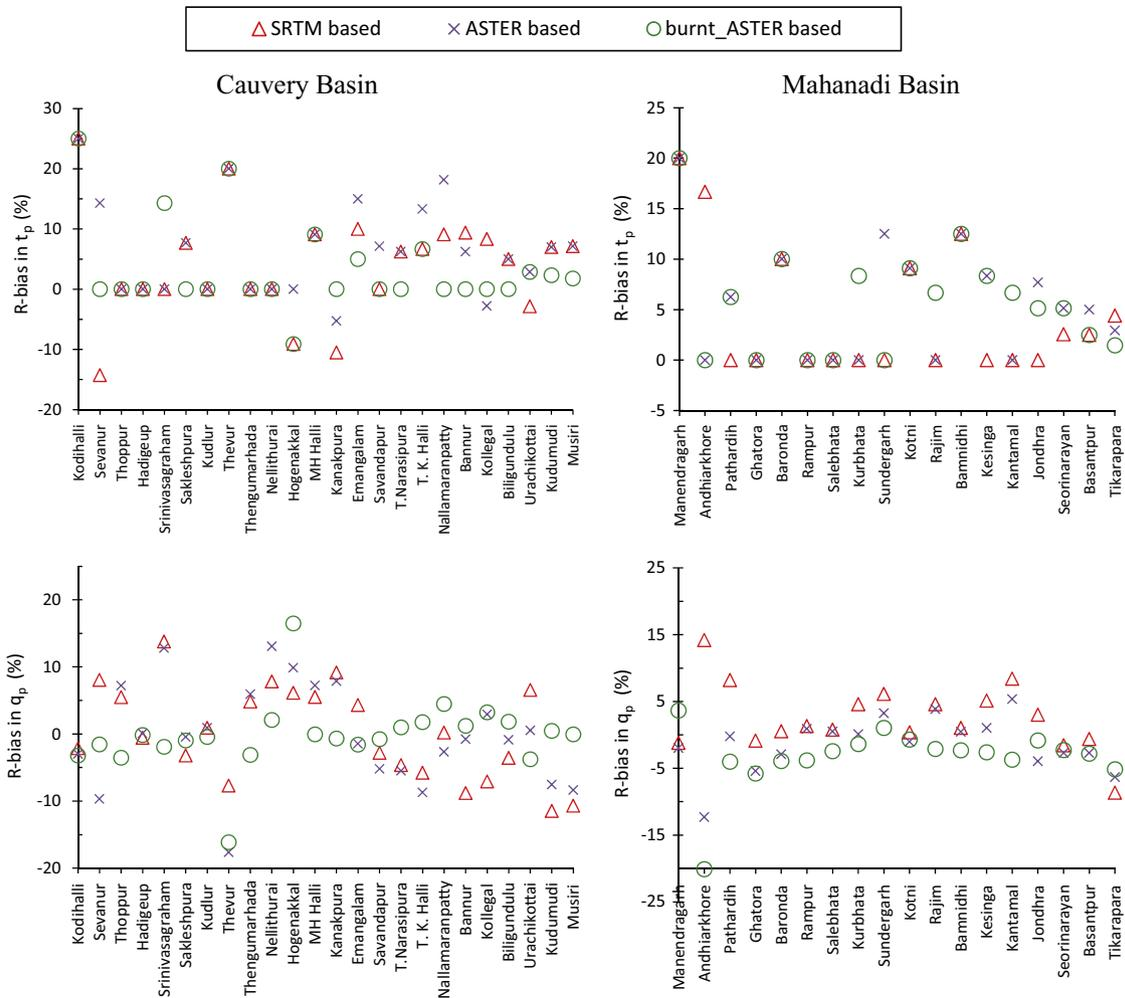
Fig. 10. Comparison of  $t_p$  (in hours) and  $q_p$  (in  $h^{-1}$ ) of E-GIUHs derived based on original SRTM and ASTER DEMs, and burnt ASTER DEM with respect to  $t_p$  and  $q_p$  of burnt SRTM DEM.
