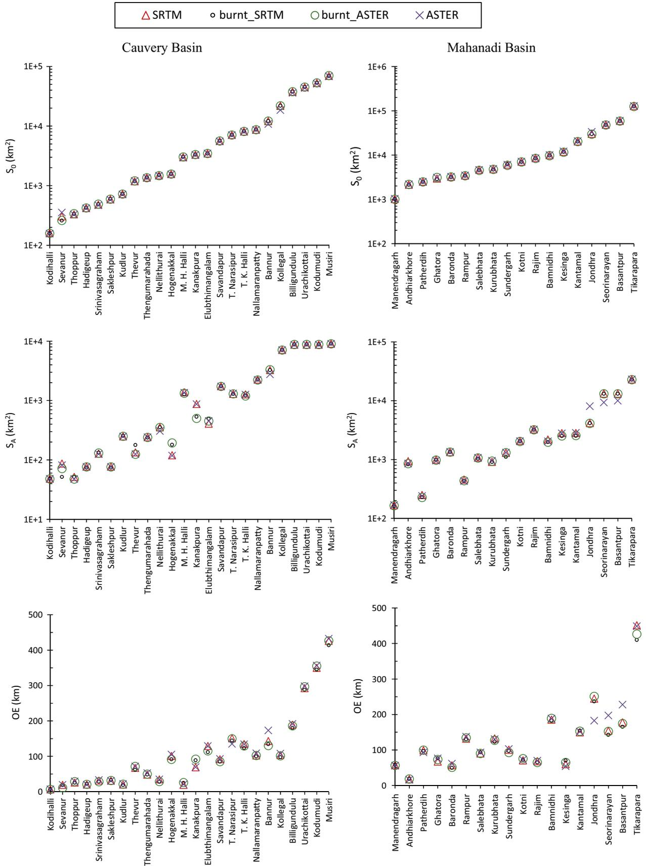
Fig. 7. Comparison of morphometric properties of channel networks extracted based on original and burnt SRTM and ASTER DEMs.
