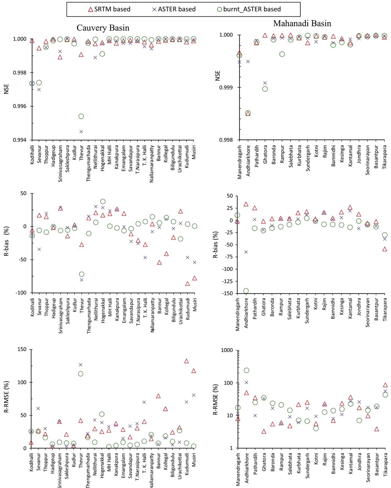
Fig. 11. Comparison of E-GIUHs derived based on original SRTM and ASTER DEMs, and burnt ASTER DEM with respect to burnt SRTM DEM.
