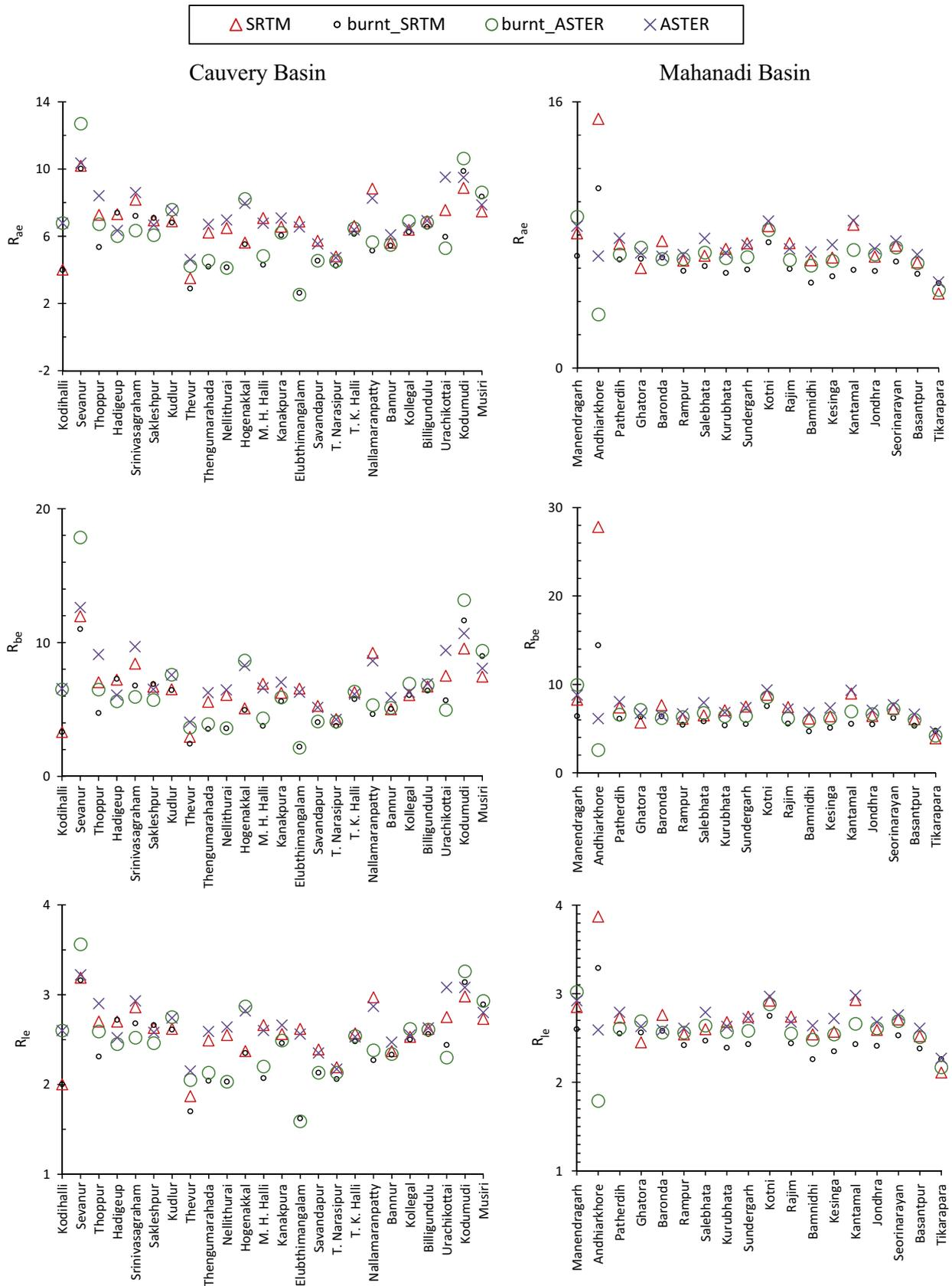
Fig. 8. Comparison of equivalent H-S ratios and equivalent length of highest order stream for channel networks extracted based on original and burnt SRTM and ASTER DEMs.
