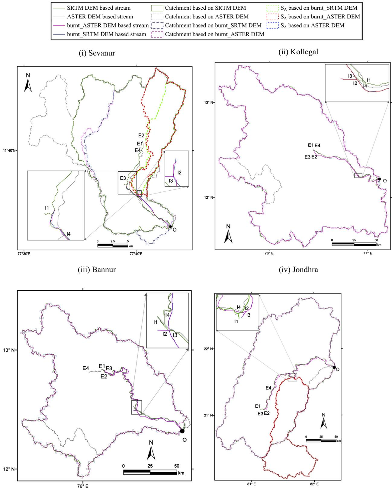
**Fig. 9.** Catchment boundary and morphometric descriptors corresponding to original and burnt SRTM and ASTER DEMs. O is catchment outlet; (OE1, I1), (OE2, I2), (OE3, I3) and (OE4, I4) denote total stream length (in km) and first bifurcation node corresponding to SRTM, burnt SRTM, burnt ASTER and ASTER DEMs respectively when  $S = S_A$ . The inset figure shows magnified view of first bifurcation nodes corresponding to various DEMs.
