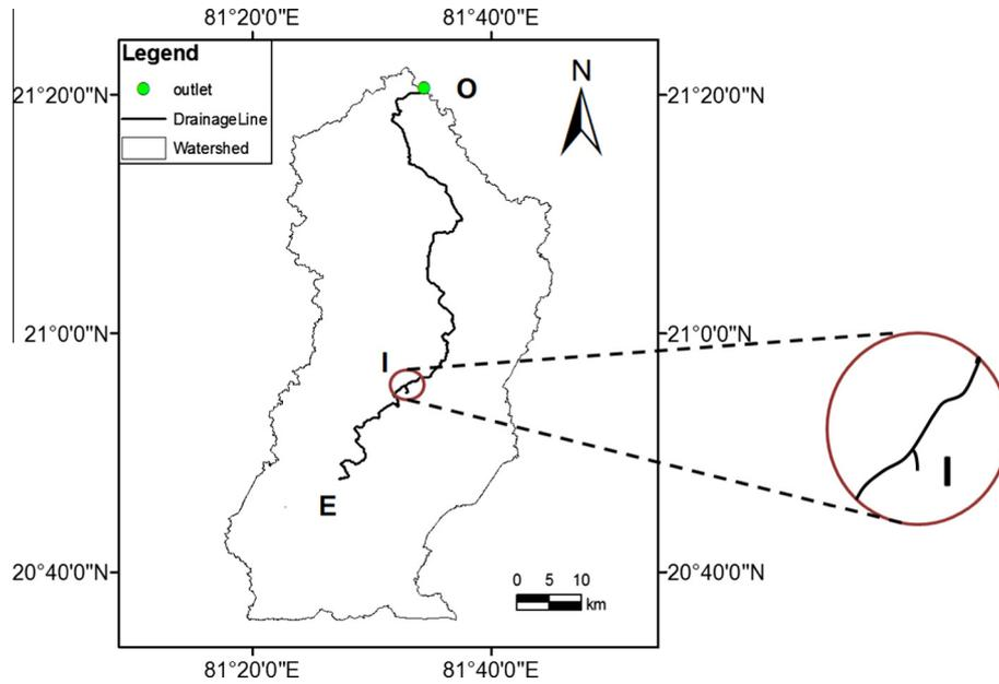
**Fig. 2.** A typical channel network for the case where threshold area  $S$  is equal to  $S_A$  (in  $\text{km}^2$ ). First bifurcation node begins at point 'I', O is outlet for the catchment, and OE is total length of the channel network (in km). The inset figure shows magnified view of first bifurcation node.
