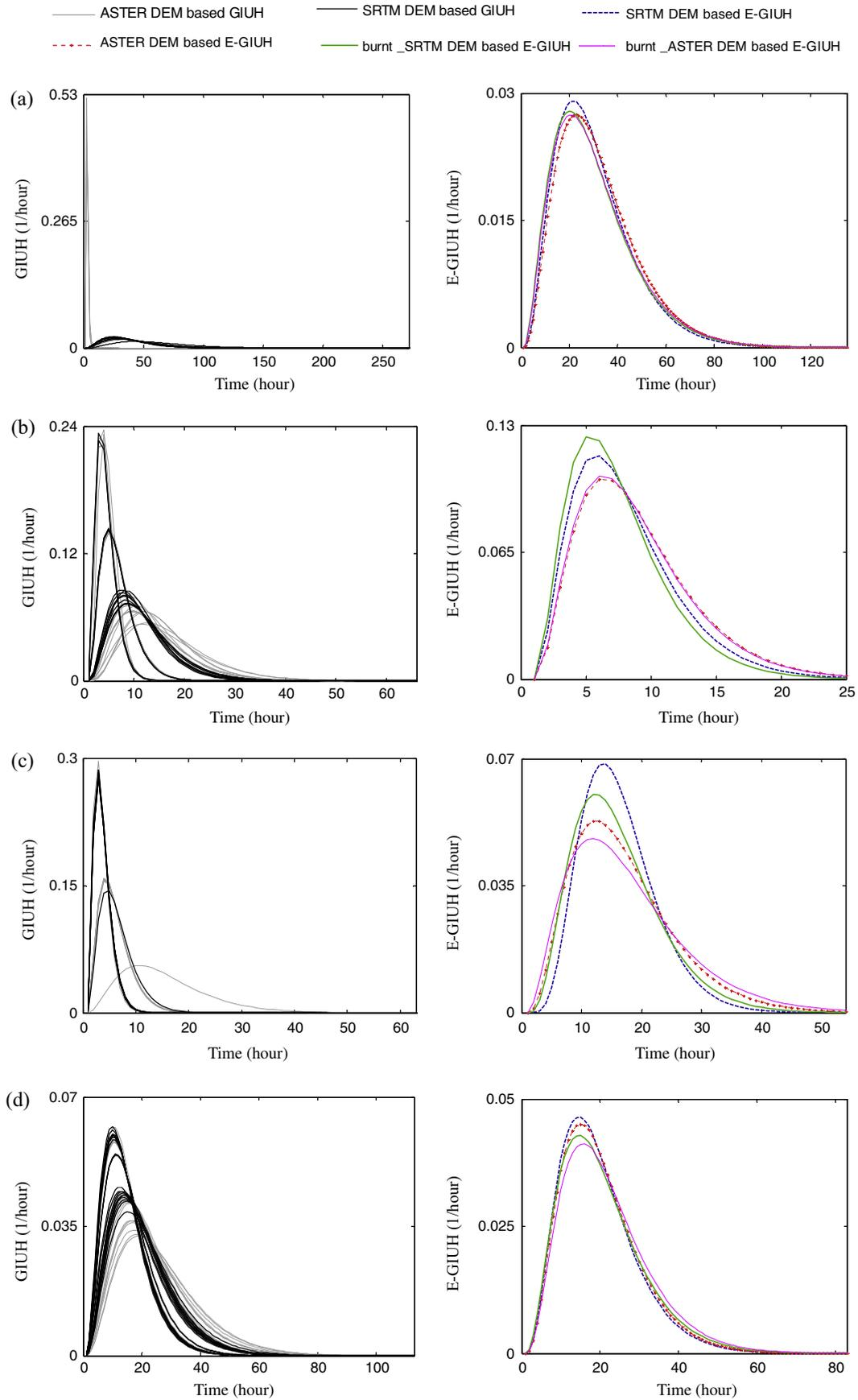
**Fig. 4.** GIUHs and E-GIUHs constructed for stream networks demarcated using 90 m resolution original and burnt SRTM DEM, and 30 m resolution original and burnt ASTER DEM for (a) Emangalam, and (b) Thevur catchments in Cauvery basin, and for (c) Andhiarkhore, and (d) Kantamal catchments in Mahanadi basin.
