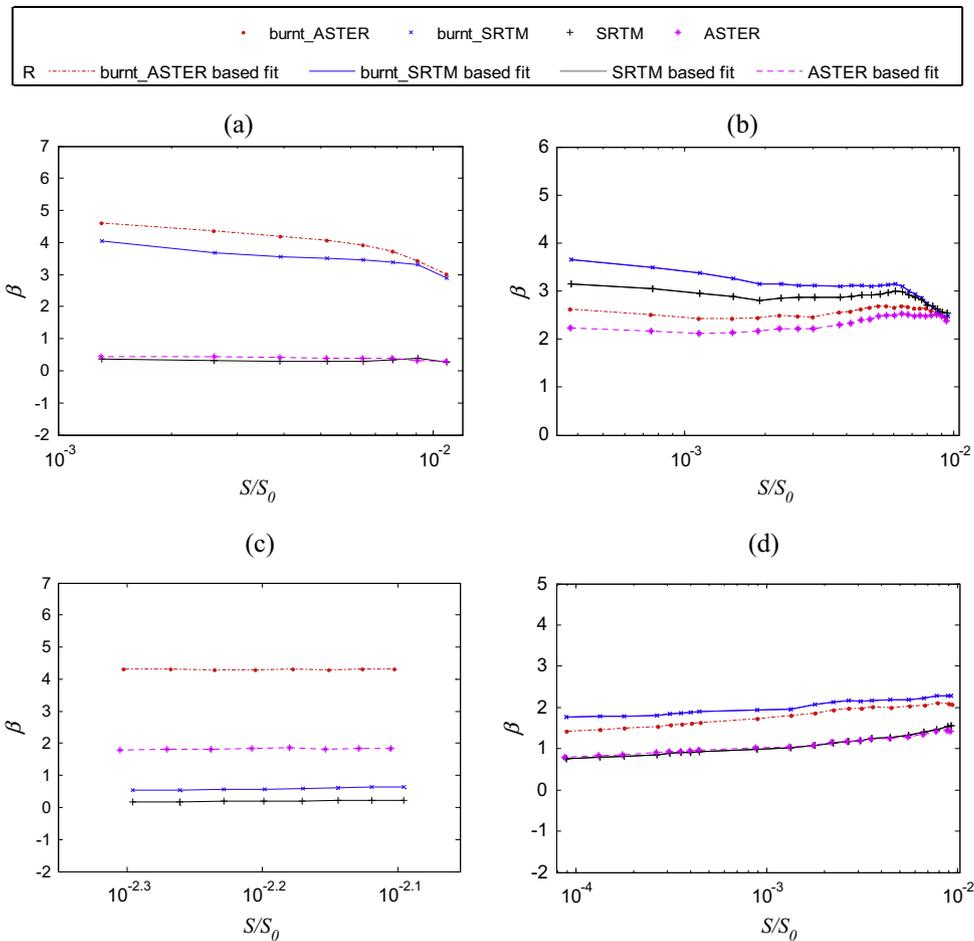
**Fig. 6.** Plots prepared to verify variation in  $\beta$  (dimensionless) value with respect to  $(S/S_0)$  (dimensionless) for (a) Emangalam, and (b) Thevur catchments in Cauvery basin, and for (c) Andhiarkhore, and (d) Kantamal catchments in Mahanadi basin.
