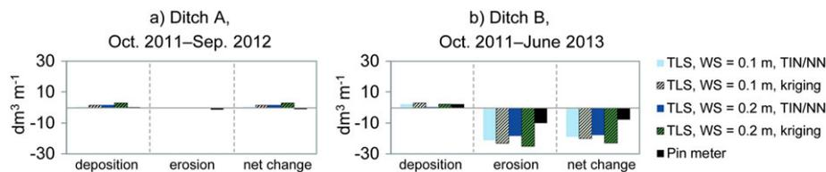
**Figure 8.** Statistically significant (at 68% confidence level) net increase (deposition) and decrease (erosion) of volumes calculated from terrestrial laser scanning (TLS) data using window sizes (WS) of 0.1 and 0.2 m (with TIN/NN and kriging methods) and from pin meter data for Ditch A with thick peat layer (a) and Ditch B with thin peat layer (b).
