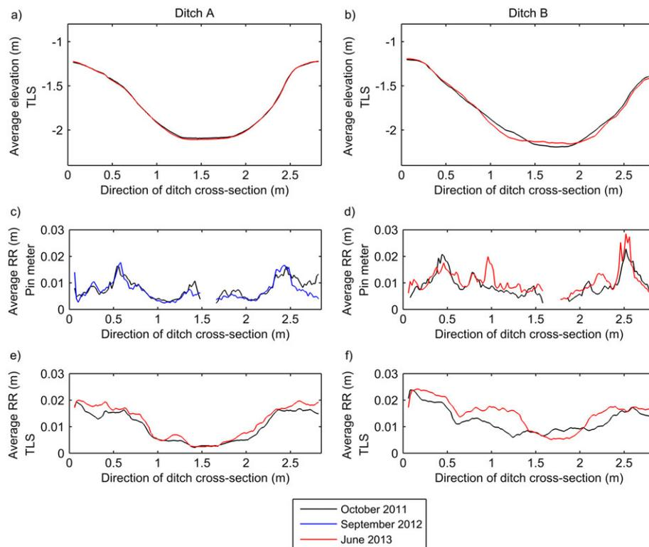
**Figure 10.** The average cross-sections defined by TLS (a–b) and variation in the average random roughness (RR) calculated for Ditch A with thick peat layer and Ditch B with thin peat layer from pin meter (c–d) and TLS data (e–f).
