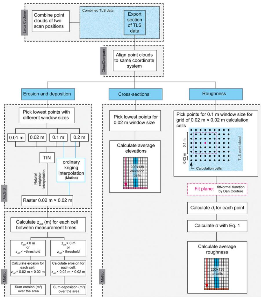
**Figure 4.** Steps used in calculating erosion, deposition, cross-sections, and roughness of the ditches from TLS data. Notation:  $z_{diff}$  is the difference in z-coordinate between the measurement times,  $d_i$  is the distance from a point to the fitted plane, and  $\sigma$  is the standard deviation of the  $d_i$ .
