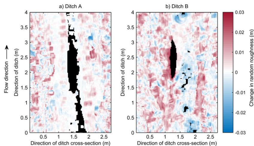
**Figure 11.** The spatial distribution of changes in random roughness from October 2011 to June 2013 calculated for Ditch A with thick peat layer (a) and Ditch B with thin peat layer (b). Black colour represents the areas with no available data.
