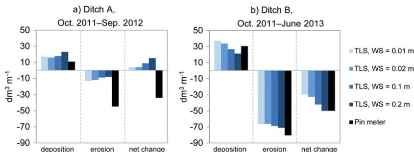
**Figure 7.** Net increase (deposition) and decrease (erosion) of volumes calculated from terrestrial laser scanning (TLS) data with varying window sizes (WS) with the TIN/NN method and from pin meter data for Ditch A with thick peat layer (a) and Ditch B with thin peat layer (b).
