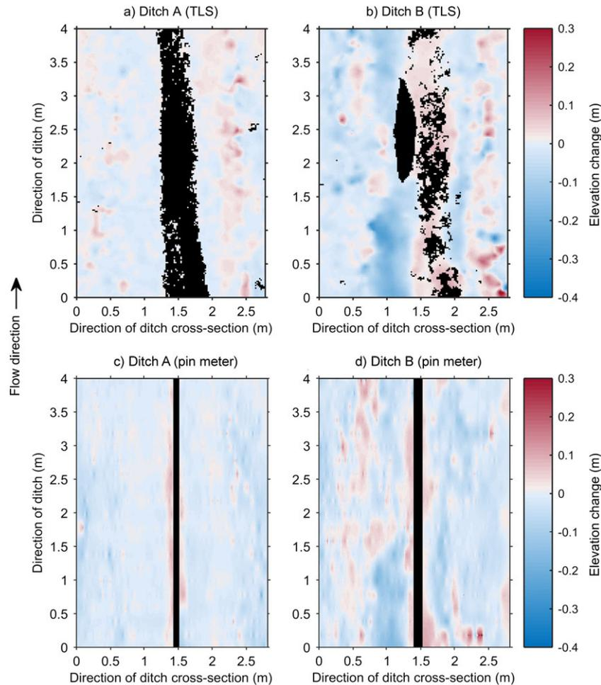
**Figure 6.** Erosion (blue) and deposition (red) calculated from TLS data (with TIN/NN method) with window size 0.1 m (a–b) and interpolated pin meter data (c–d) between October 2011 and September 2012 for Ditch A with thick peat layer and between October 2011 and June 2013 for Ditch B with thin peat layer. Black colour represents areas with no data.
