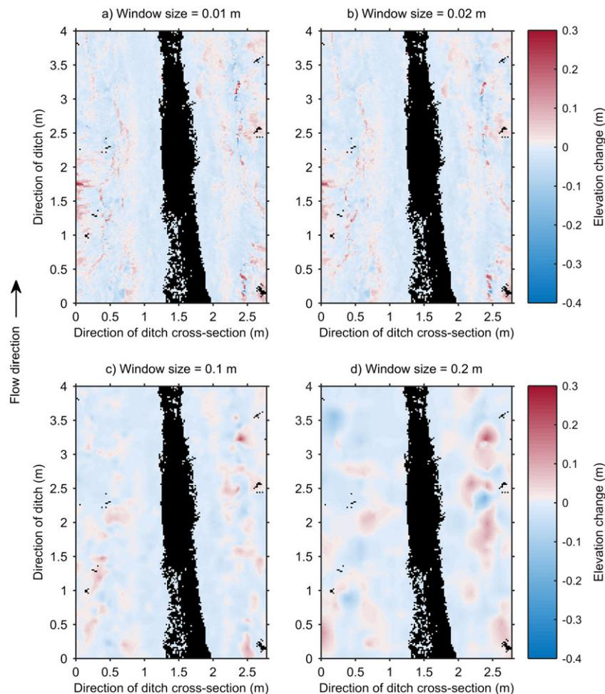
**Figure 5.** Spatial visualization of erosion (blue) and deposition (red) between October 2011 and June 2013 for a peat ditch (A in Figure 1) calculated with the TIN/NN method using different window sizes: 0.01 m (a), 0.02 m (b), 0.1 m (c), and 0.2 m (d). Black colour represents areas with no TLS data.
