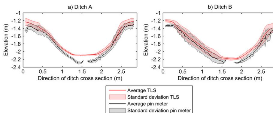
**Figure 9.** Average cross-section ( $\pm$  standard deviation) calculated from pin meter data and lowest elevation points picked for 0.02 m  $\times$  0.02 m grid from TLS data at Ditch A (a) and Ditch B (b) in October 2011.
