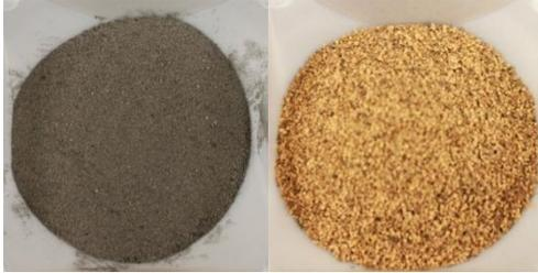
Figure 3: Graphite (Left), Nut Shells (Right)
