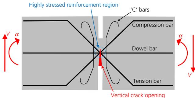
Figure 4. Schematic hinge joint under applied shear force ( $V$ ) and rotation ( $\alpha$ )
