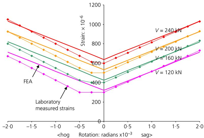
Figure 8. 3D FEA compared to physical model for peak axial strain in tension hinge bar
