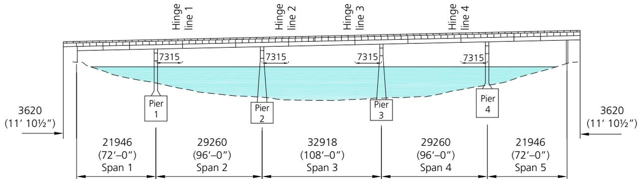
Figure 1. General arrangement details of the underbridge. Elevation looking upstream (dimensions in mm)
