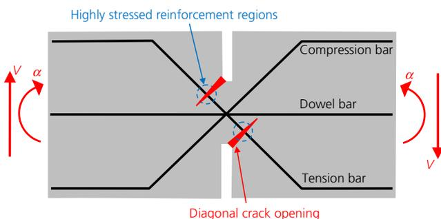
Figure 5. Schematic hinge joint under ultimate shear load typical of research for development of BA93/09
