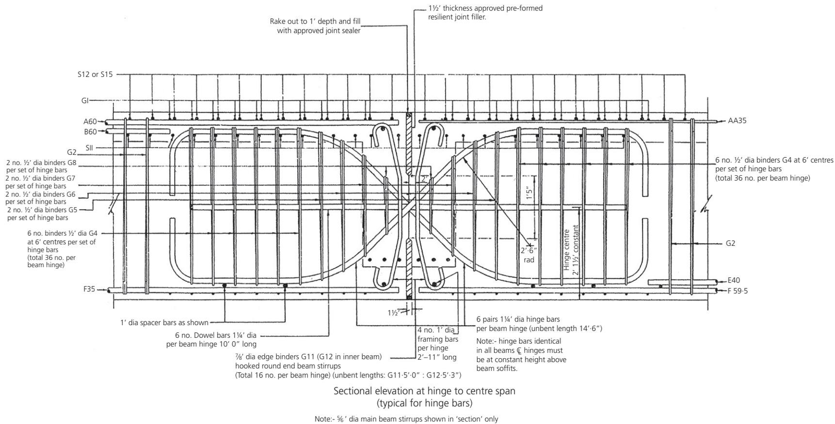
Figure 3. Hinge joint details
