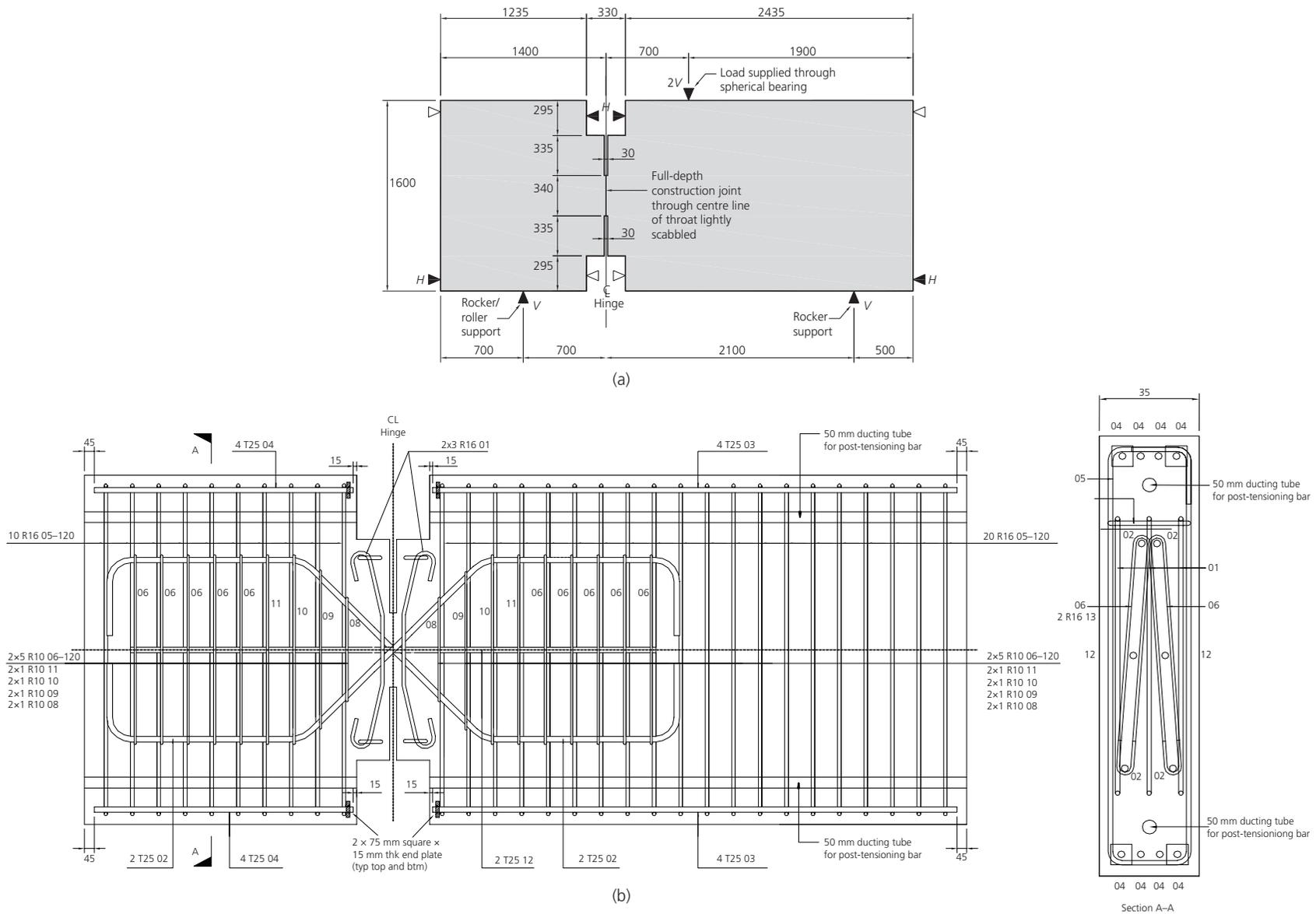
Figure 6. Hinge model (a) outline and (b) reinforcement details
