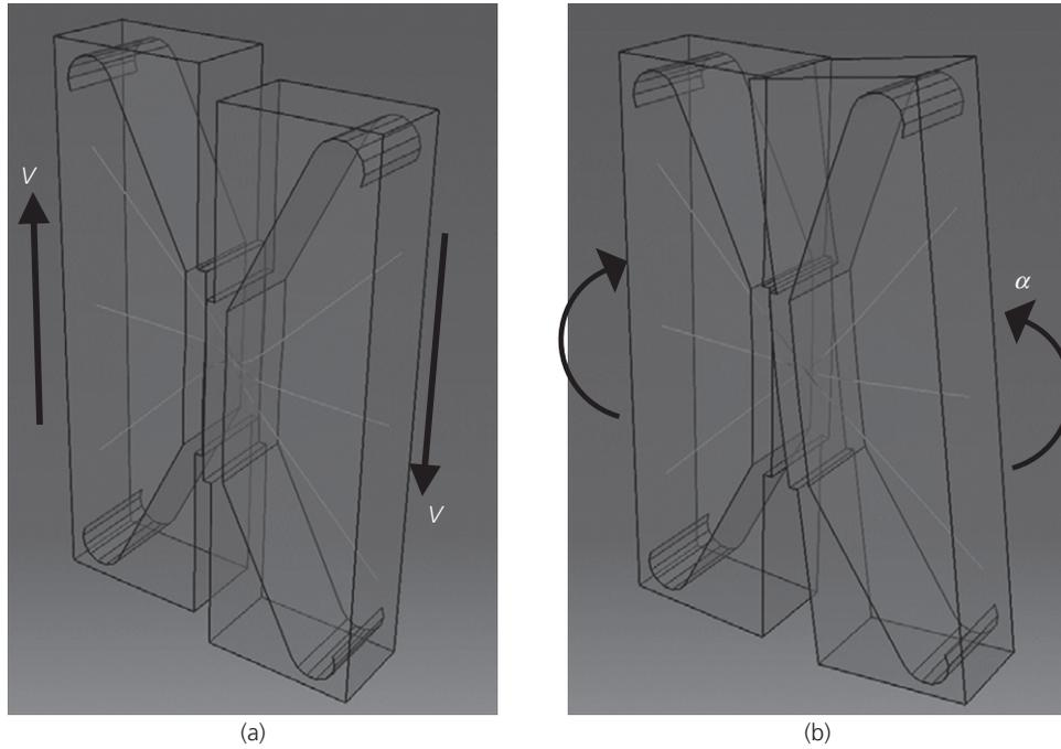
Figure 7. Three-dimensional finite-element model subject to (a) shear ( $V$ ) and (b) rotation ( $\alpha$ )
