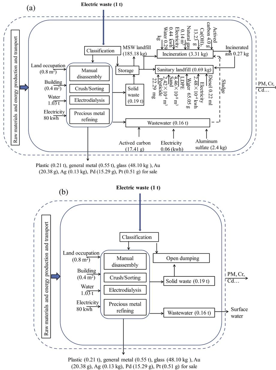
Fig. 1. System boundary and mass flow (a) ET-D scenario; (b) ET-ND scenario.
