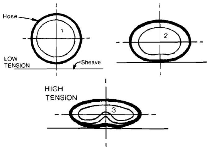
Fig. 7. Hydraulic hose failure by sheaving (Bryant, 1990).
