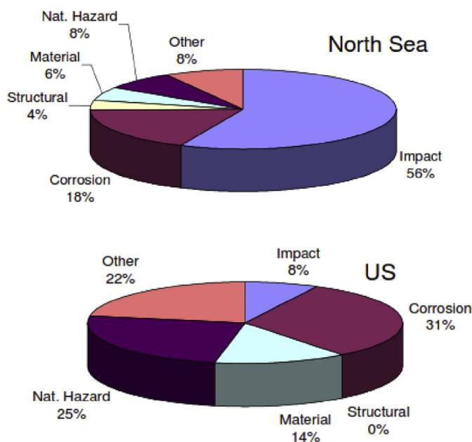
Fig. 1. Offshore pipeline failures (Stadie-Frohbs and Lampe, 2013).
