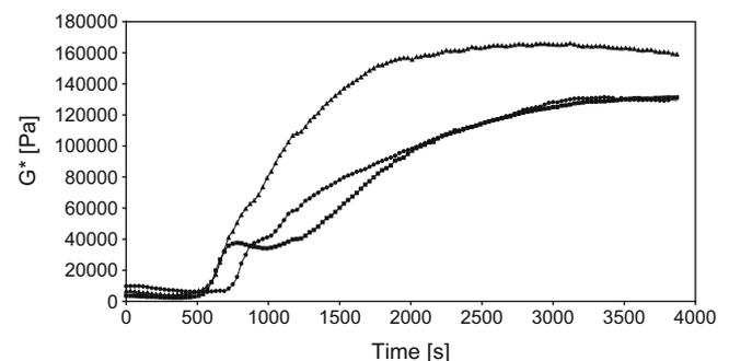
**Fig. 2.** Changes in complex moduli of GFD 1, GFD 2 and CGD during heating and cooling (40 – 95 – 40 °C), (◆ – GFD 2, ▲ – GFD 1, ■ – CGD).
