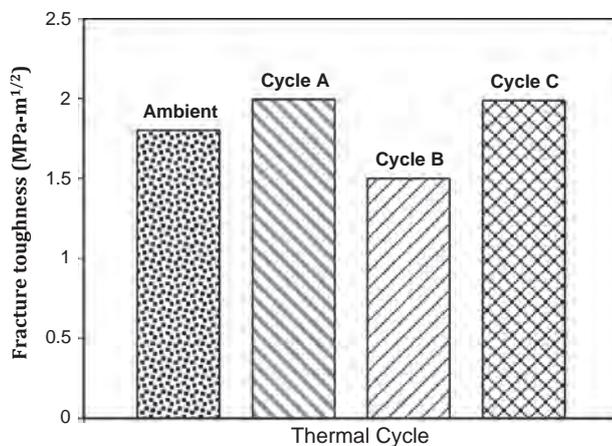
**Fig. 6.** Comparison of fracture toughness of PC under three thermal cycles and ambient conditions.
