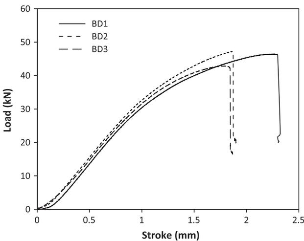
Fig. 5. Load–displacement curves of BD specimens under thermal cycle-B.
