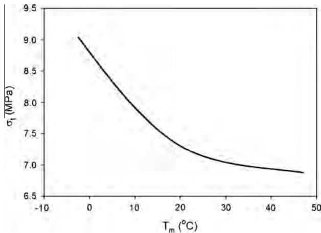
Fig. 11. Empirical relationship between the tensile strength and the mean temperature ( $T_m$ ) obtained for the tested PC materials at different thermal cycles.
