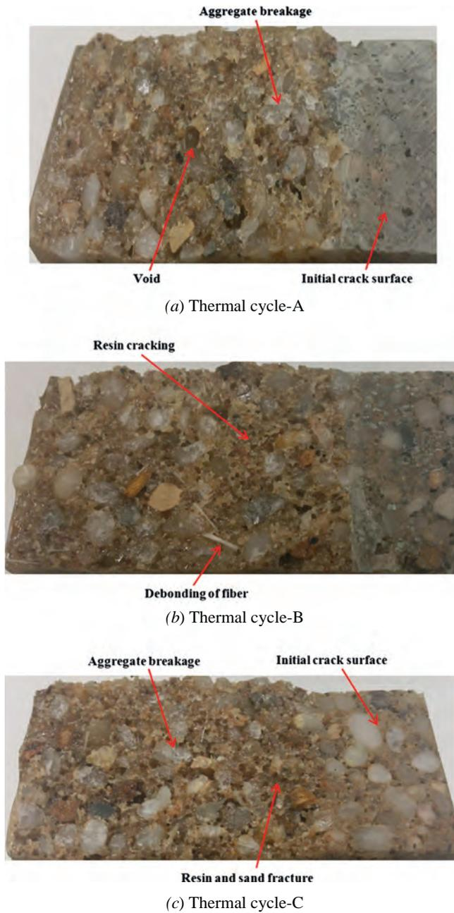
Fig. 9. Typical fracture surfaces observed for the SENB specimens tested at different thermal cycles.
