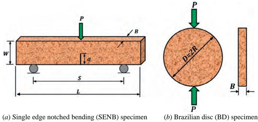
Fig. 1. Configurations of SENB and BD specimens.
