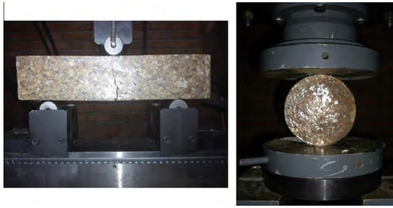
Fig. 3. SENB and BD test setup.
