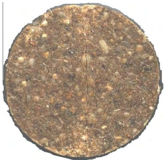
**Fig. 8.** Typical fracture trajectory observed for a BD specimen made of PC material.
