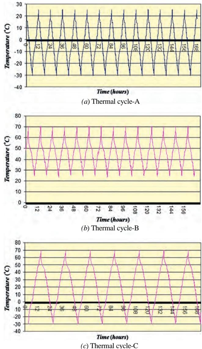
Fig. 2. Profiles of thermal cycles applied to the PC test samples.
