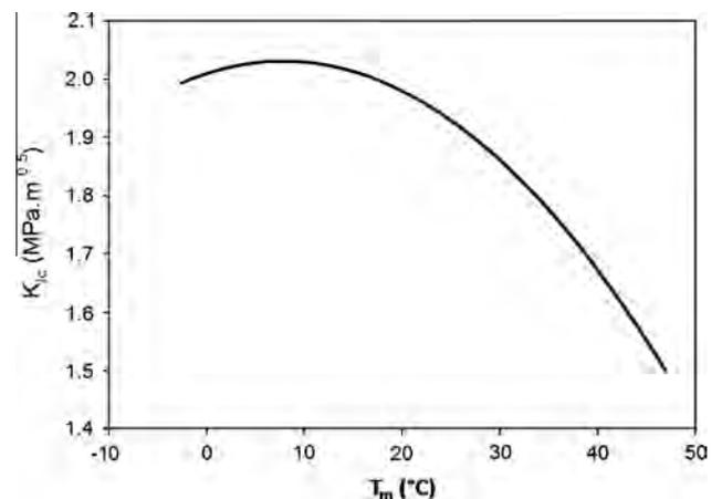
Fig. 10. Empirical relationship between the fracture toughness and the mean temperature ( $T_m$ ) obtained for the tested PC materials at different thermal cycles.
