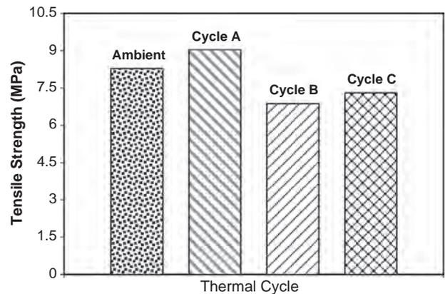
**Fig. 7.** Tensile strength of PC material tested under ambient conditions and three thermal cycles-A, -B and -C.
