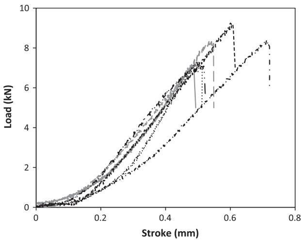
Fig. 4. Load–displacement curves of SENB specimens under thermal cycle-A.
