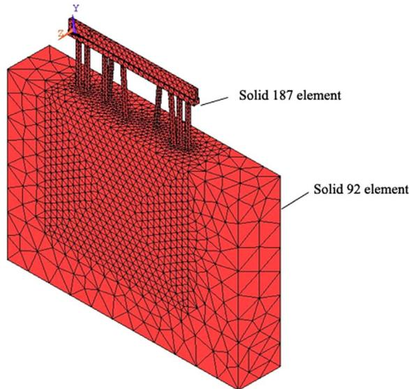
Fig. 13. Meshed finite element model of the bent structure with two pairs of batter piles.
