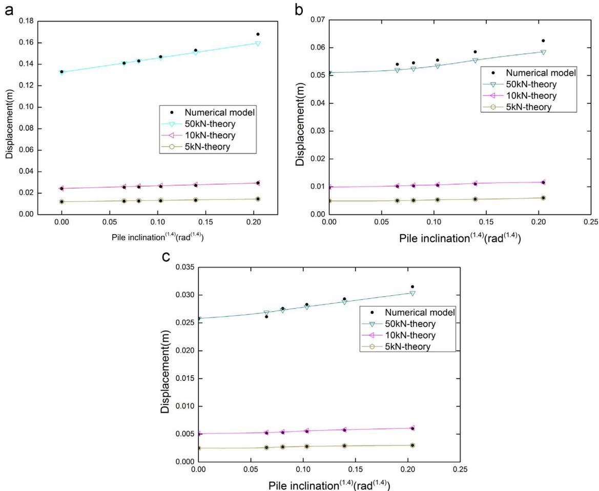
Fig. 5. Comparison of theoretical calculation and numerical simulation results. (a) Pile with square section of  $0.6\text{ m} \times 0.6\text{ m}$ . (b) Pile with square section of  $0.8\text{ m} \times 0.8\text{ m}$ . (c) Pile with square section of  $1.0\text{ m} \times 1.0\text{ m}$ .
