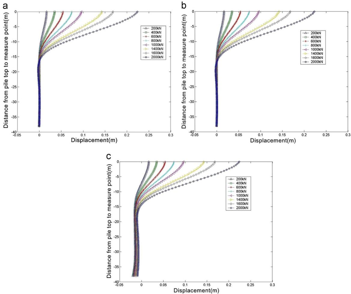
Fig. 14. Distribution profile of horizontal displacements along piles. (a) Pile #1 of bent with two pairs of batter piles. (b) Pile #4 of bent with two pairs of batter piles. (c) Pile #6 of bent with two pairs of batter piles.
