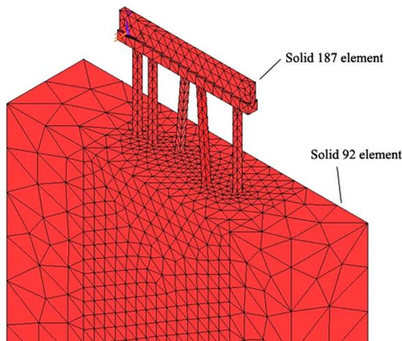
Fig. 10. Meshed finite element model of the bent structure with a pair of batter piles.
