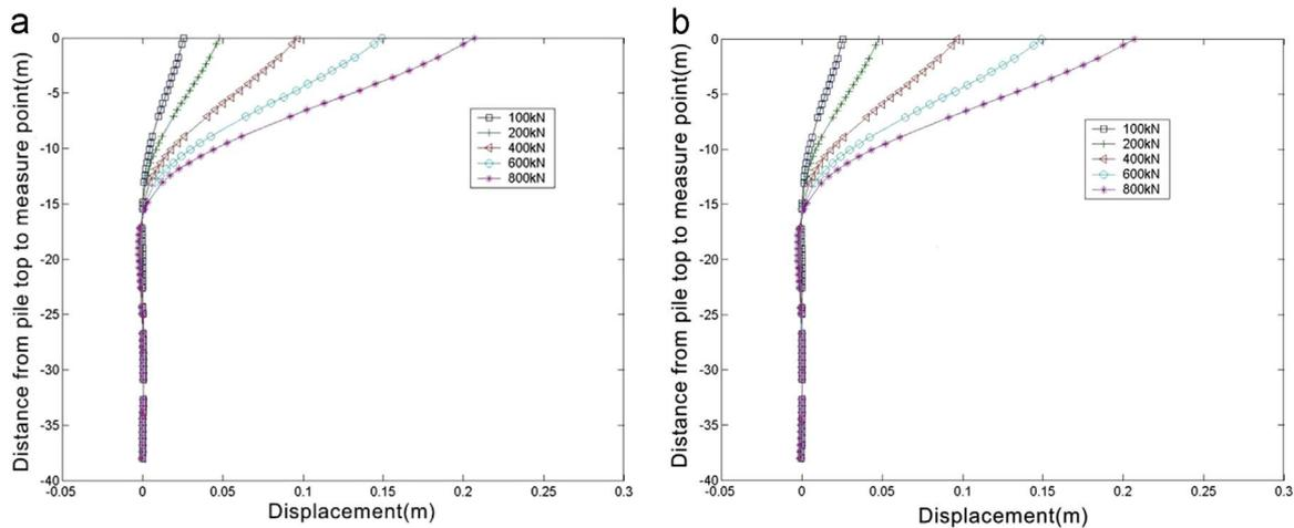
Fig. 8. Displacement profiles of Piles #1 and #3 subjected to lateral load. (a) Pile #1 of bent with all plumb piles. (b) Pile #3 of bent with all plumb piles.
