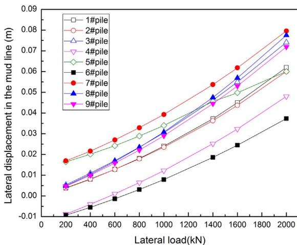
Fig. 15. Lateral load-displacement relation for bent with two pairs of batter piles.
