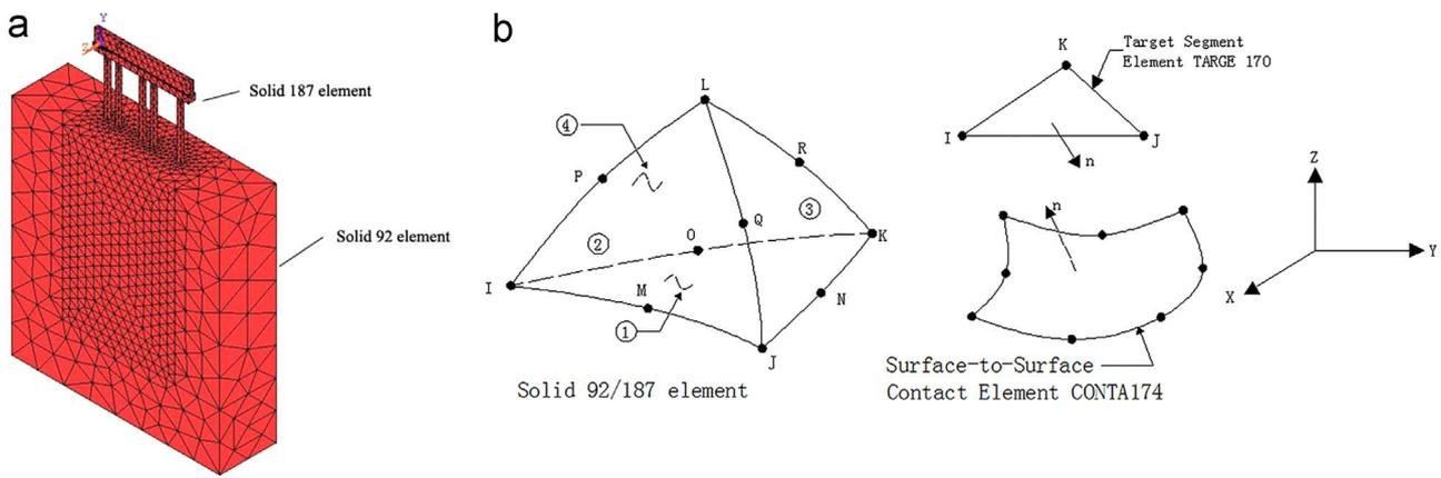
Fig. 7. (a) Element division of bent with all plumb piles. (b) Geometry of solid elements and contact surface elements.
