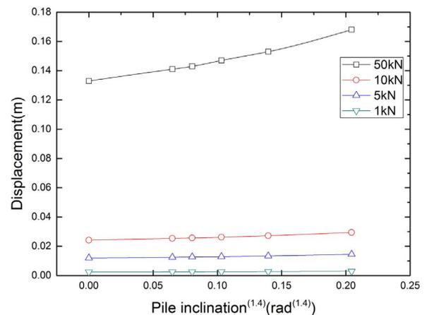
Fig. 3. Displacement of pile top vs. pile inclination angle. (The exponent m here is equal to 1.4).
