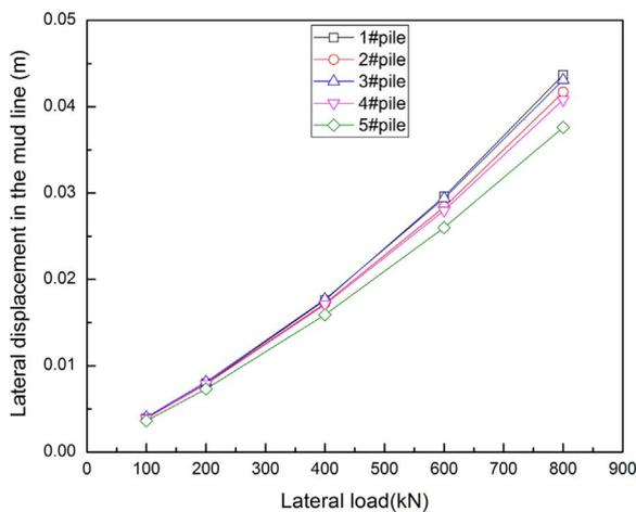
Fig. 9. Lateral load-displacement relation of bent with all plumb piles.
