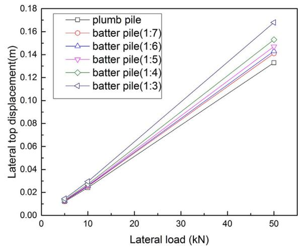
Fig. 6. Lateral load-displacement relation for single pile with varying slope.
