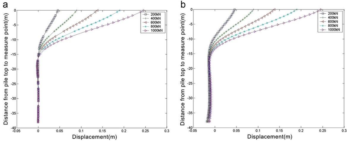
Fig. 11. The distribution law of displacements along piles in vertical direction. (a) Pile #1 of bent with a pair of batter piles. (b) Pile #3 of bent with a pair of batter piles.
