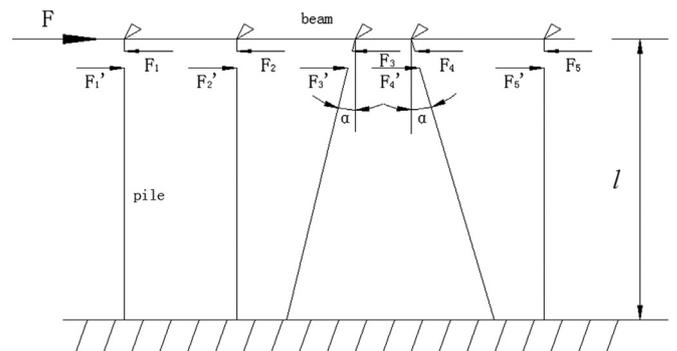
Fig. 16. Free body diagram of bent model.
