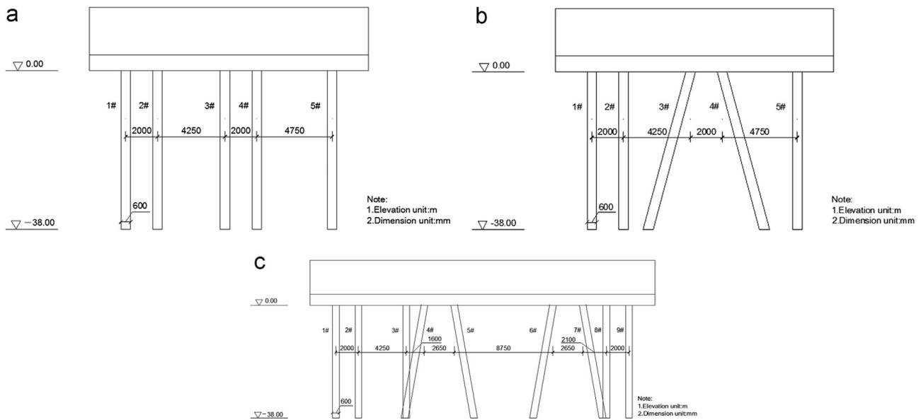
Fig. 2. Bent structure layout and dimensions. (a). Layout of bent structure with all plumb piles. (b). Layout of bent structure with one pair of batter piles. (c). Layout of bent structure with two pairs of batter piles.
