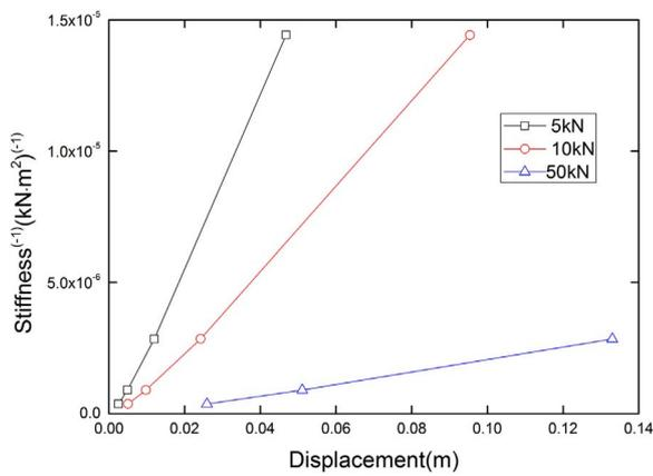
Fig. 4. The relationship between the stiffness and the horizontal displacement of plumb pile.
