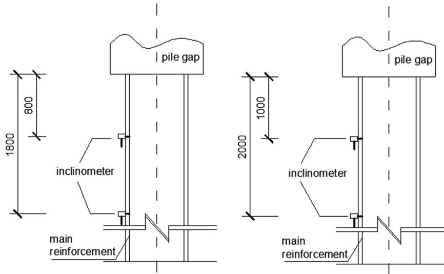
**Fig. 17.** Arrangement of inclinometers along the pile body (unit: mm).
