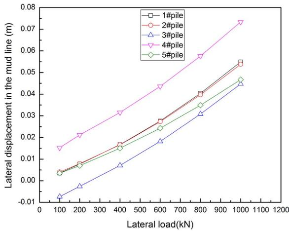
Fig. 12. Lateral load-displacement relation of bent with a pair of batter piles.
