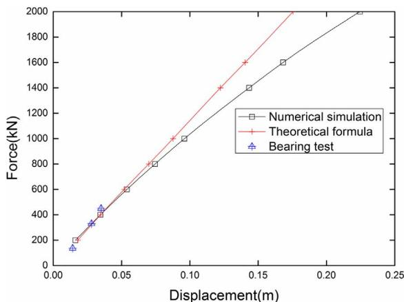
**Fig. 18.** Comparison of numerical simulation, theoretical formula and experimental (berthing test) results.
