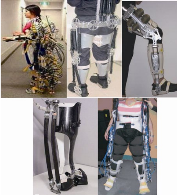
Fig. 6. Experimental devices driven by pneumatic system
