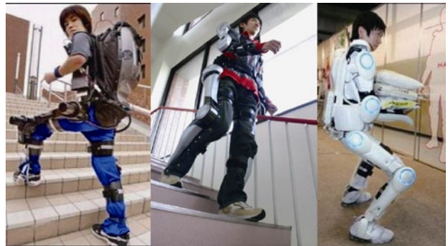
Fig. 4. HAL series of the University of Tsukuba
