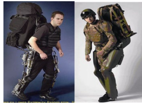
Fig. 1. BLEEX of the University of California, Berkeley
