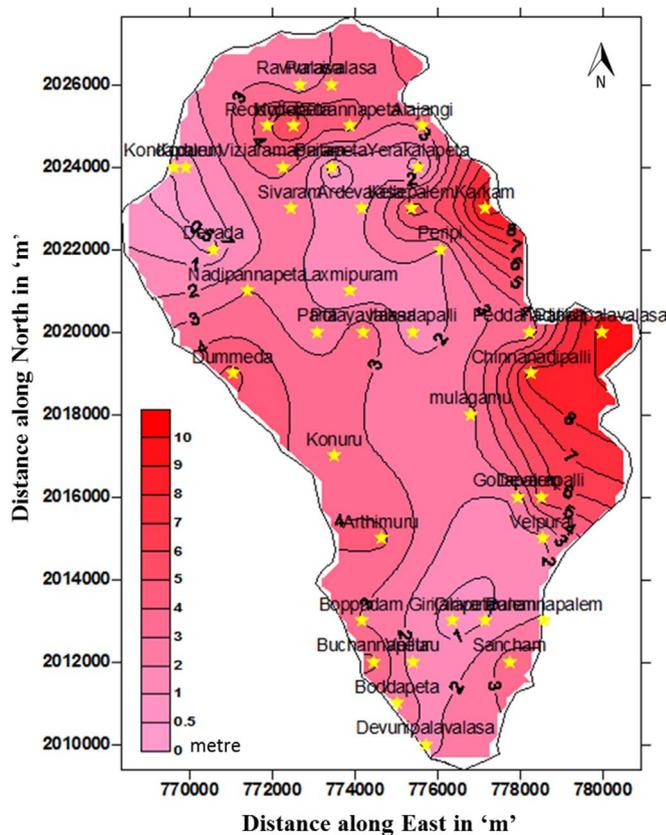
Fig. 7. Contour map of groundwater fluctuations of KRSB during the year 2015.
