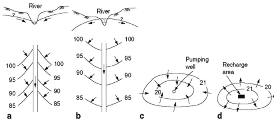
Fig. 8. Features exhibited by water table contour maps: (a) Effluent Seepage (b) Influent Seepage (c) Groundwater Depression (d) Groundwater Mound (Singhal and Gupta, 2010).
