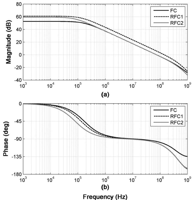
Fig. 6. Amplifiers AC response. (a) Magnitude. (b) Phase.
