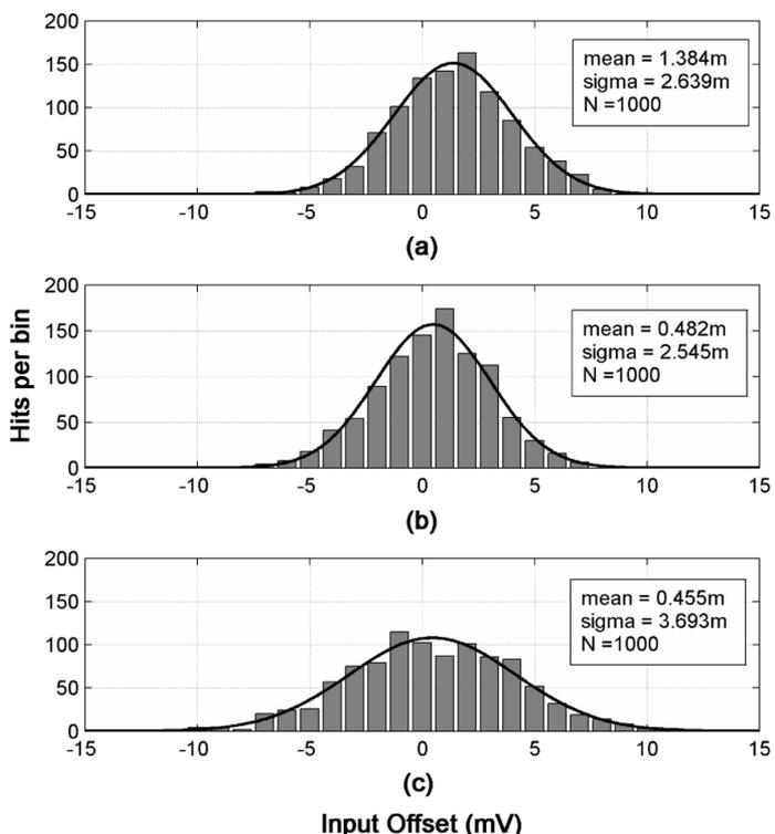
Fig. 11. Input offset distributions. (a) Conventional folded cascode. (b) Recycling folded cascode 1. (c) Recycling folded cascode 2.
