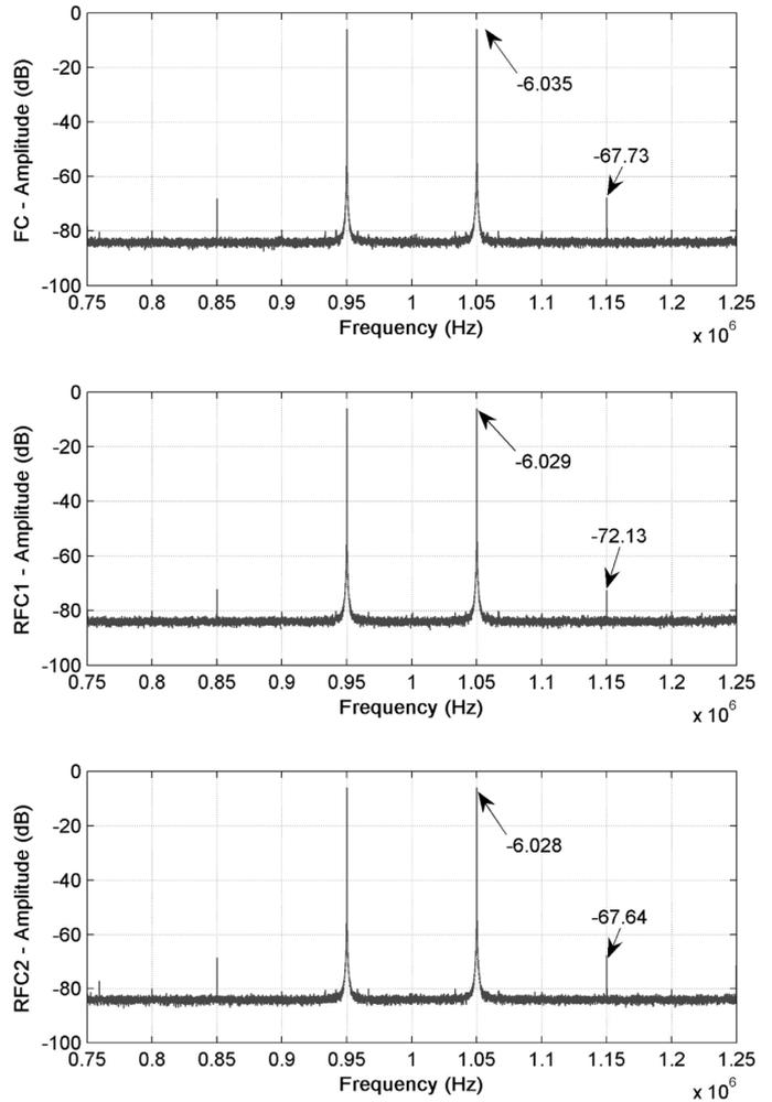
Fig. 9. Two tone FFT spectrums of the FC, RFC1 and RFC2 for a 1 V<sub>pp</sub> signal centered at 1 MHz and separated by 100 kHz.
