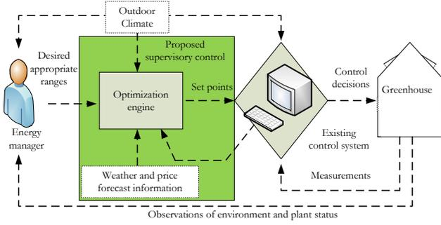
Fig. 2. Greenhouse existing and proposed supervisory control architecture.
