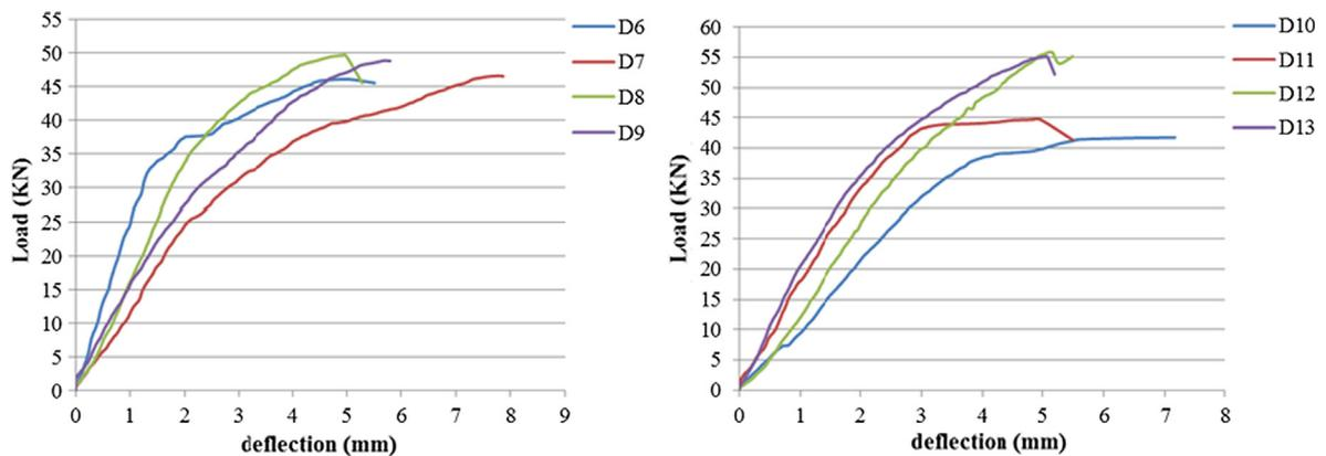
Fig. 6. Load–deflection curves for repaired slabs.
