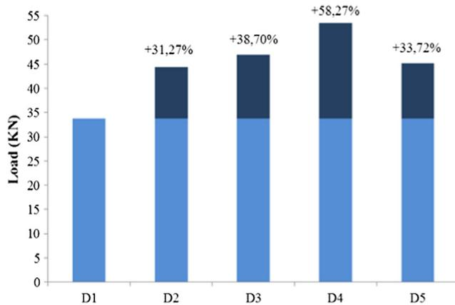
**Fig. 2.** Ultimate load of reinforced slabs.
