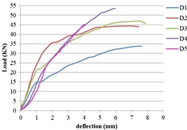
Fig. 5. Load–deflection curves for control and reinforced slabs.
