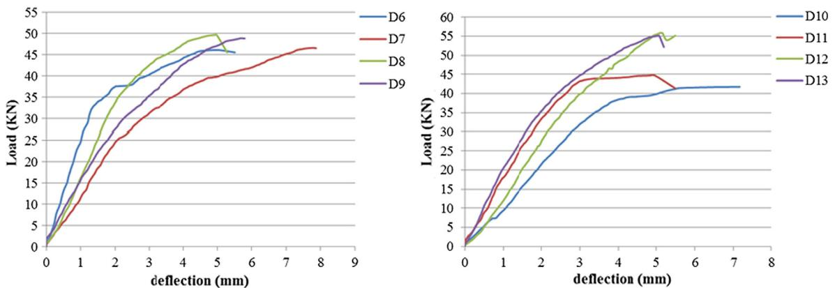
Fig. 6. Load–deflection curves for repaired slabs.
