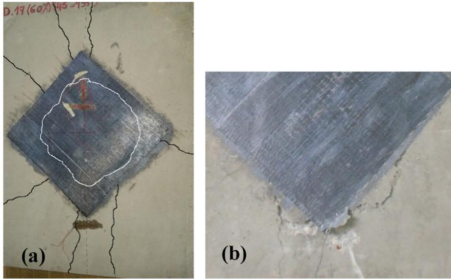
Fig. 4. (a) Failure of repaired slab (b) debonding of CFRP with concrete.
