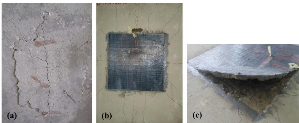
**Fig. 3.** (a) Failure of control slabs (b) failure of reinforced slab (c) debonding of CFRP.
