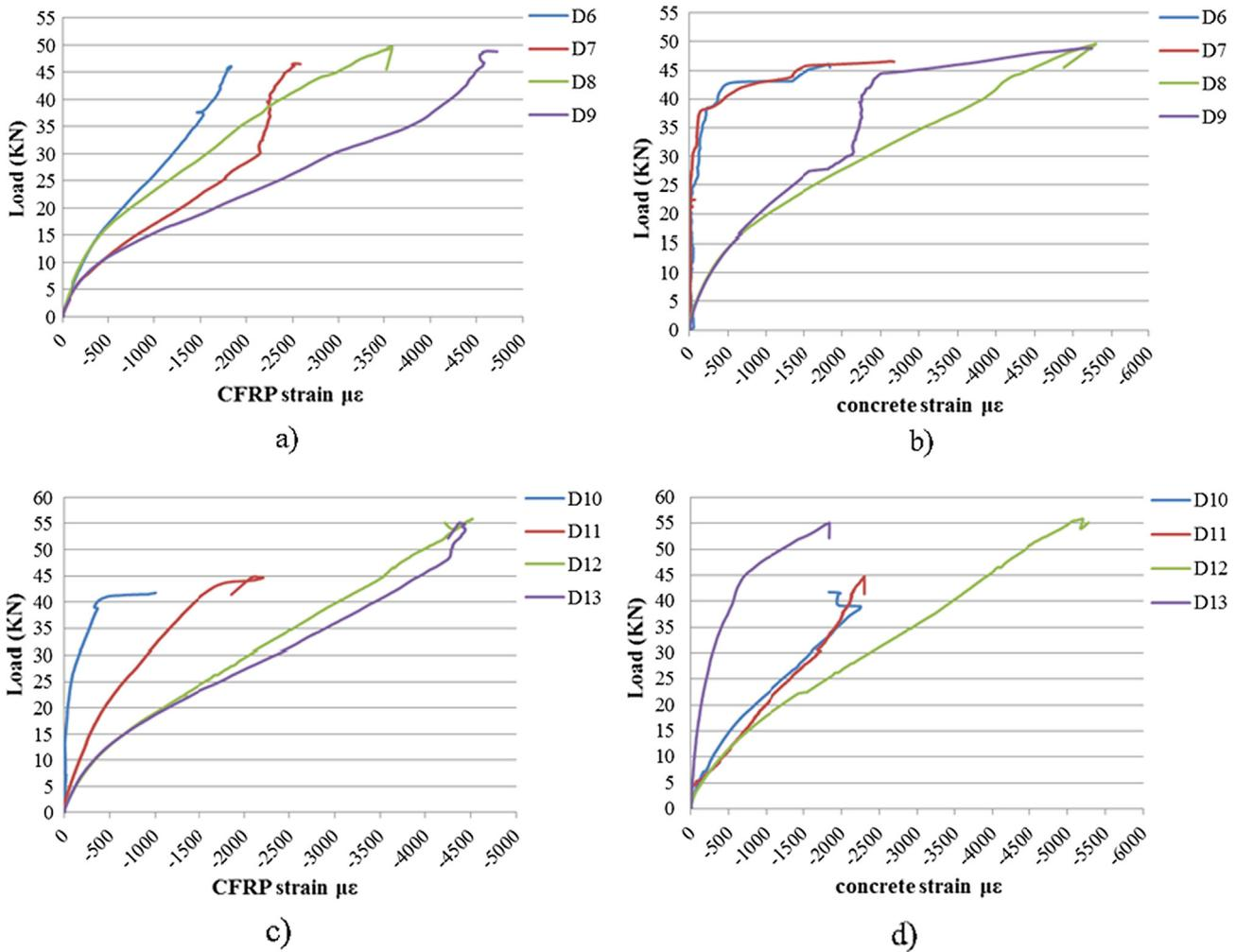
Fig. 8. CFRP and concrete strain of repaired slabs (preload slabs).
