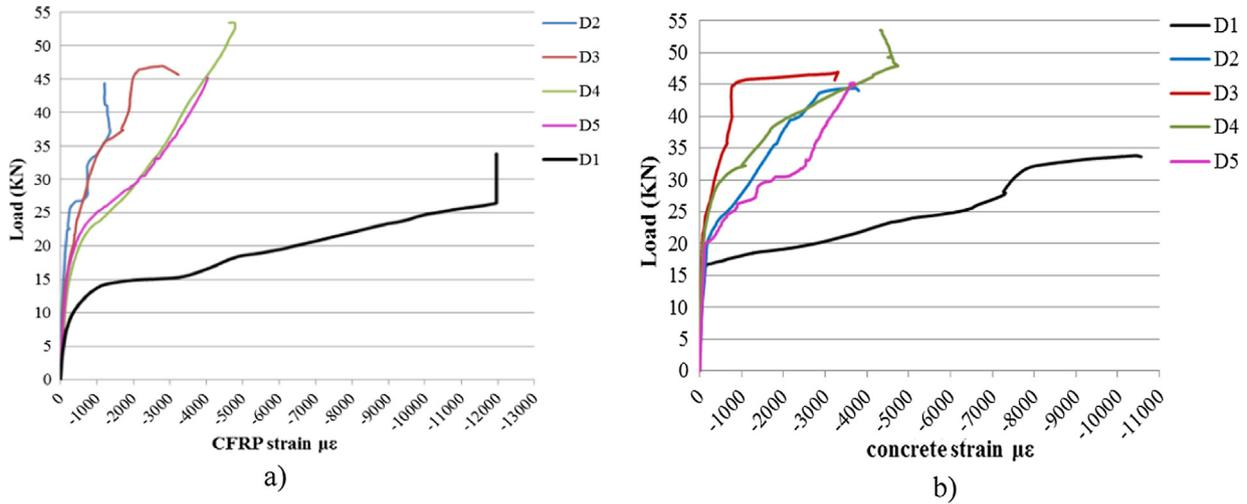
Fig. 7. (a) CFRP strain of control and reinforced slabs. (b) Concrete strain of control and reinforced slabs.
