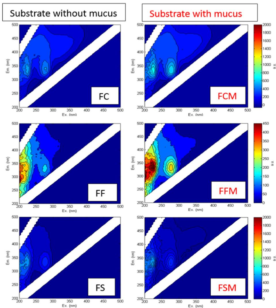
**Fig. 1.** Fluorescence excitation–emission matrix spectra of dissolved organic matter from final products with and without earthworms' mucus in the three decomposition systems. 'F' in each image means the final product; C, F and S pertain to the three systems of cow dung, fresh fruit and vegetable wastes and sewage sludge, respectively; 'M' represents substrates added with mucus.
