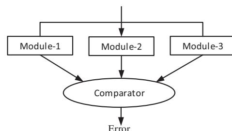
Fig. 2. Triple modular redundancy fault detection technique.
