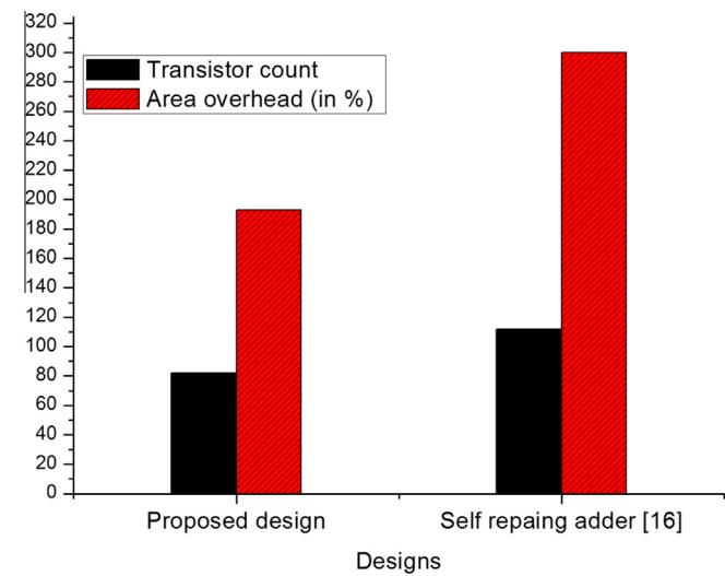
Fig. 9. Comparison of transistor count and area overhead of proposed and self repairing adder [16].
