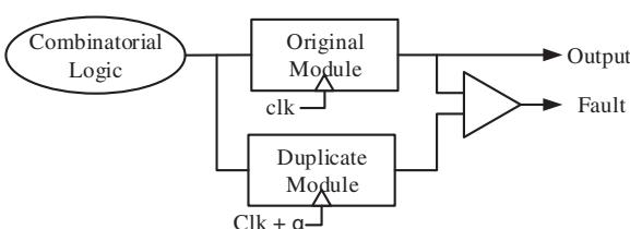
Fig. 1. Time redundancy fault detection technique.
