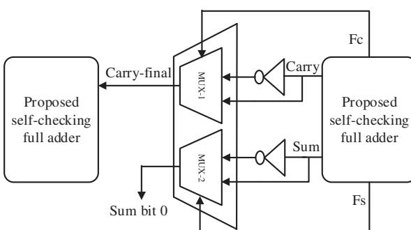
Fig. 8. Proposed self repairing full adder design.
