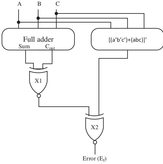
Fig. 5. Self checking full adder.
