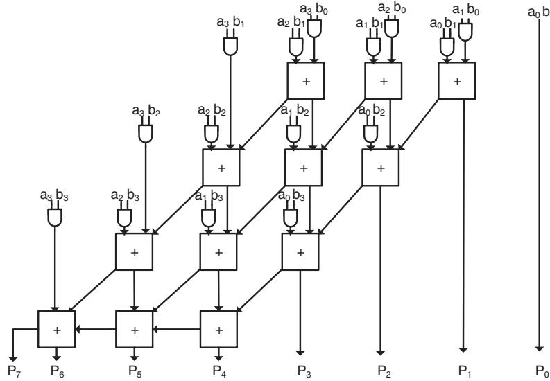
**Fig. 11.** Fault tolerant multiplier design using 1-bit proposed self repairing full adder.
