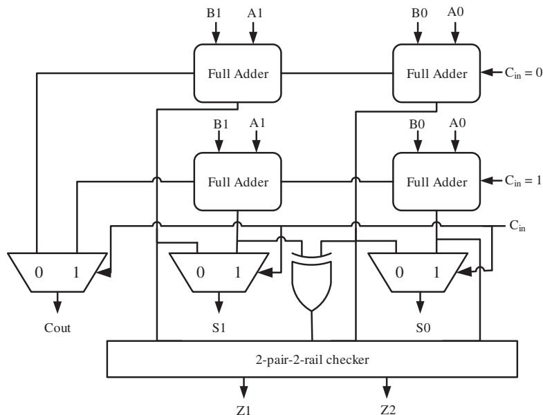
**Fig. 4.** 2-Bit self checking carry select adder.
