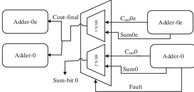
Fig. 6. Self repairing adder.
