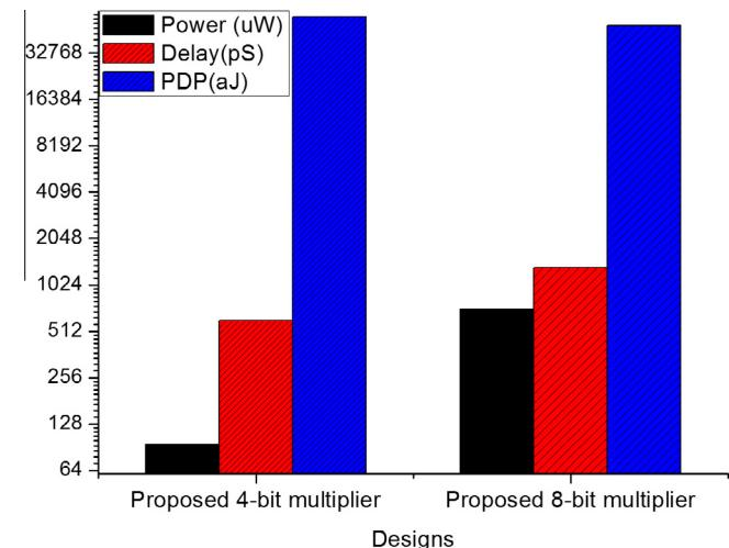
**Fig. 12.** Power, delay and PDP of 4-bit and 8-bit proposed fault tolerant multiplier.
