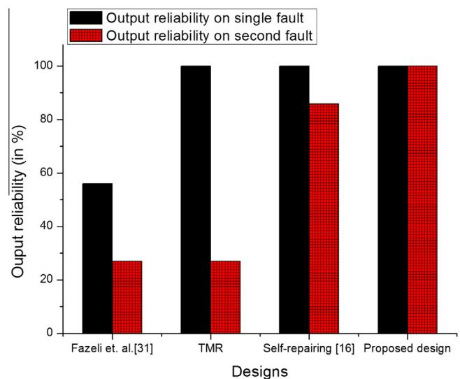
**Fig. 10.** Comparison of fault recovery and reliability of the proposed and existing designs.
