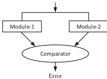
**Fig. 3.** Double modular redundancy fault detection technique.
