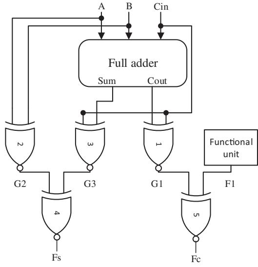
Fig. 7. Proposed self checking full adder design.
