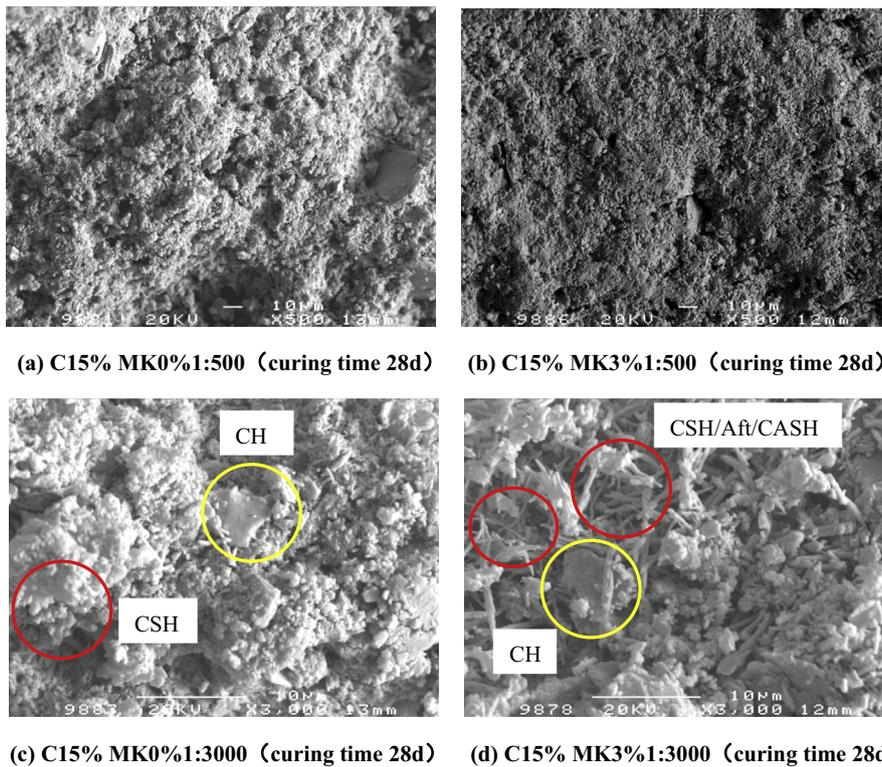
Fig. 8. SEM photos of MK-cement treated clay after 28 days of curing.
