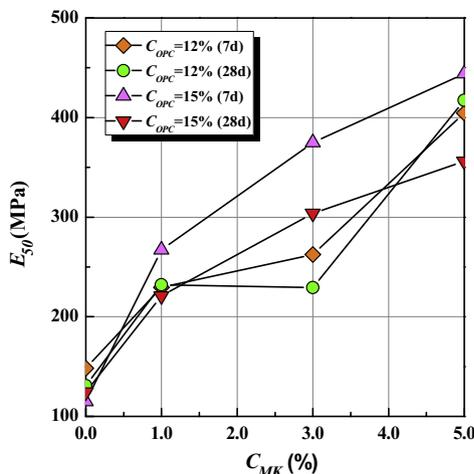
Fig. 4. Relationship between  $E_{50}$  (MPa) and MK contents (%).
