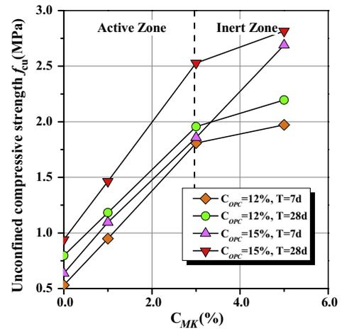
**Fig. 2.** Relationship between  $f_{cu}$  (MPa) and MK contents (%).
