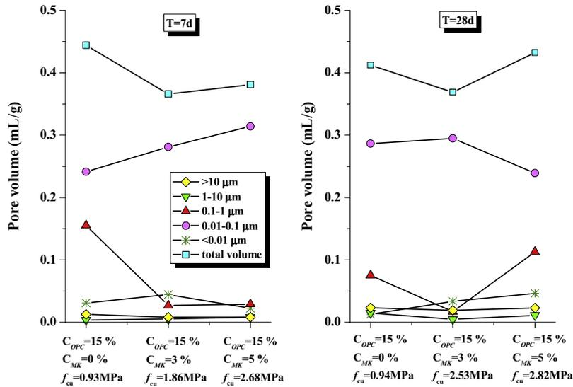
Fig. 7. Pore size distribution classified by an order of magnitude of different proportion of cement and MK.
