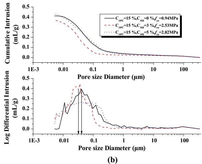
Fig. 6. Cumulative mercury intrusion and log differential intrusion vs. pore size diameter curve (a) after 7 days of curing, and (b) after 28 days of curing.
