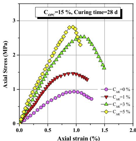
**Fig. 1.** UCT results with 15% cement after 28 days of curing.
