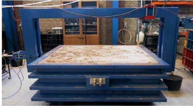
Fig. 6. Test box used for loading tests on bucket foundations.
