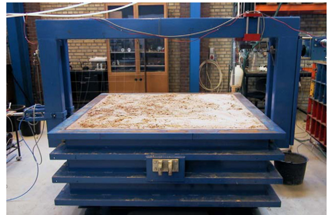
Fig. 6. Test box used for loading tests on bucket foundations.
