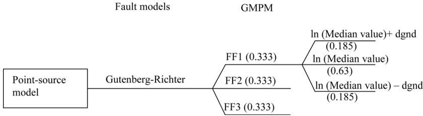
**Figure 4.** Logic tree for the PSHA procedure used by [Petersen et al. \(2008\)](#).
