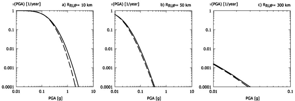
**Figure 6.** Comparison of mean hazard curves for PGA. The continuous line is the mean hazard curve computed considering the uncertainty in the regression coefficients while the dashed line is the mean hazard curve computed disregarding this uncertainty.
