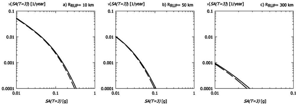
**Figure 7.** Comparison of mean hazard curves for  $SA(T=3)$ . The continuous line is the mean hazard curve computed considering the uncertainty in the regression coefficients while the dashed line is the mean hazard curve computed disregarding this uncertainty.
