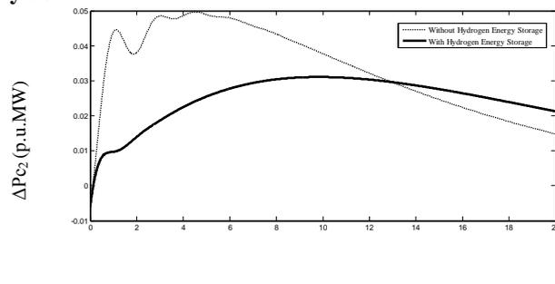
Fig.7 Dynamic responses of the frequency deviations, tie- line power deviations, and Control input deviations for TAT restructured scenario-2 (bilateral based transactions)
