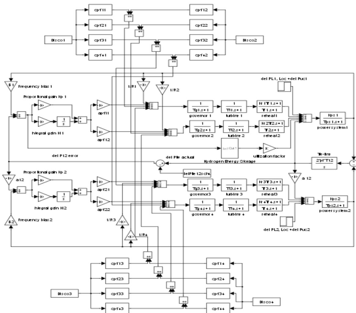
Fig. 5 Simulink model of a Two- Area Thermal Reheat Interconnected Power System (TATRIPS) in restructured environment with Hydrogen Energy Storage unit.
