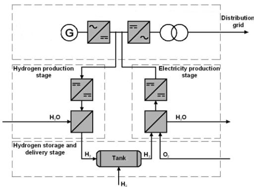
Fig 3 Block diagram of the hydrogen storage unit
