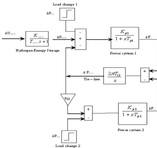
Fig. 4 Linearized reduction model for the control design
