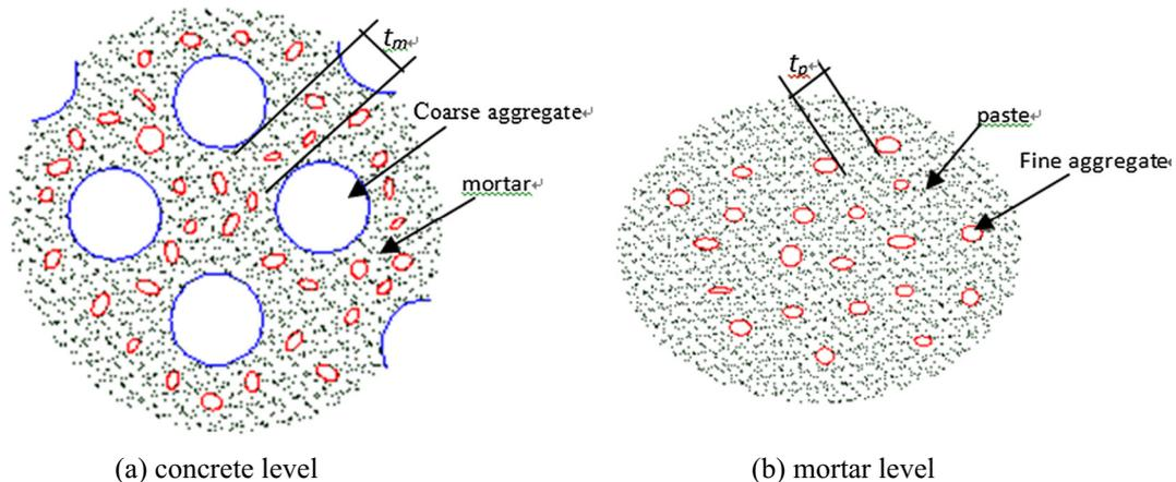
Fig. 4. Schematic diagram of physical models for concrete and mortar.
