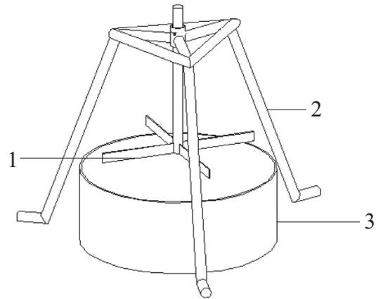
Fig. 3. Testing setup for top surface paste thickness measurement, 1 – steel testing cross, 2 – cylindrical container, 3 – bracket.
