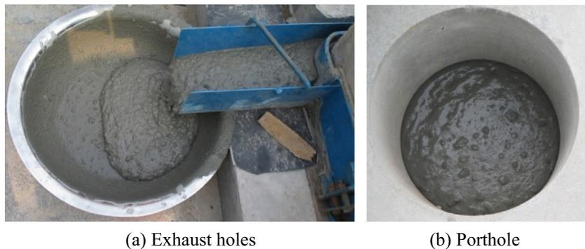
**Fig. 8.** Observation of SSFSCC from exhaust hole and porthole.
