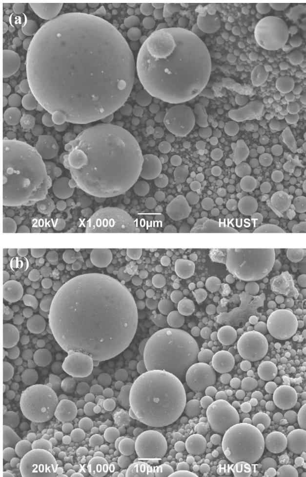
Fig. 2. SEM images of fly ash.
