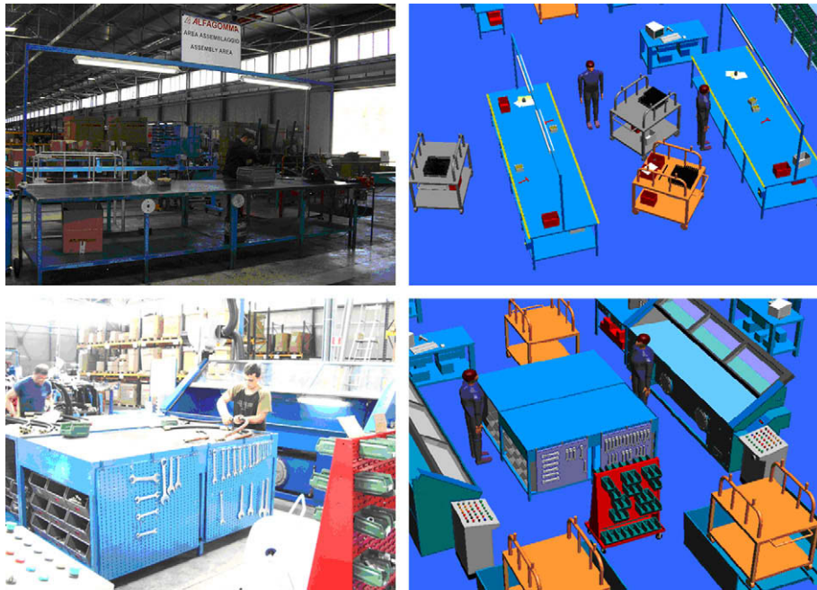
Fig. 2. Real and virtual Assembly workstation, real and virtual Pressure test workstation.
