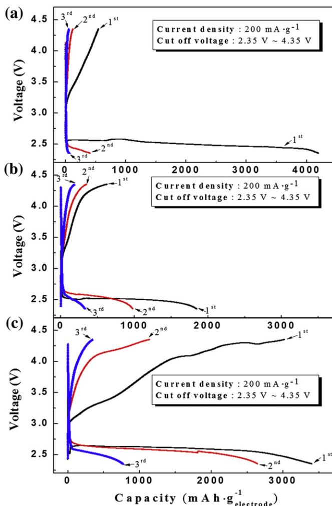
**Fig. 8.** Discharge/charge profiles of the three different electrodes for initial three cycles: (a) electrode containing plain carbon spheres as a catalyst; (b) electrode containing commercial  $\text{Co}_3\text{O}_4$  nanopowder as a catalyst; (c) electrode containing carbon-sphere/ $\text{Co}_3\text{O}_4$  nanocomposite as a catalyst (The voltage range was 4.35–2.35 V and the current density was  $200 \text{ mA g}^{-1}$ ).
