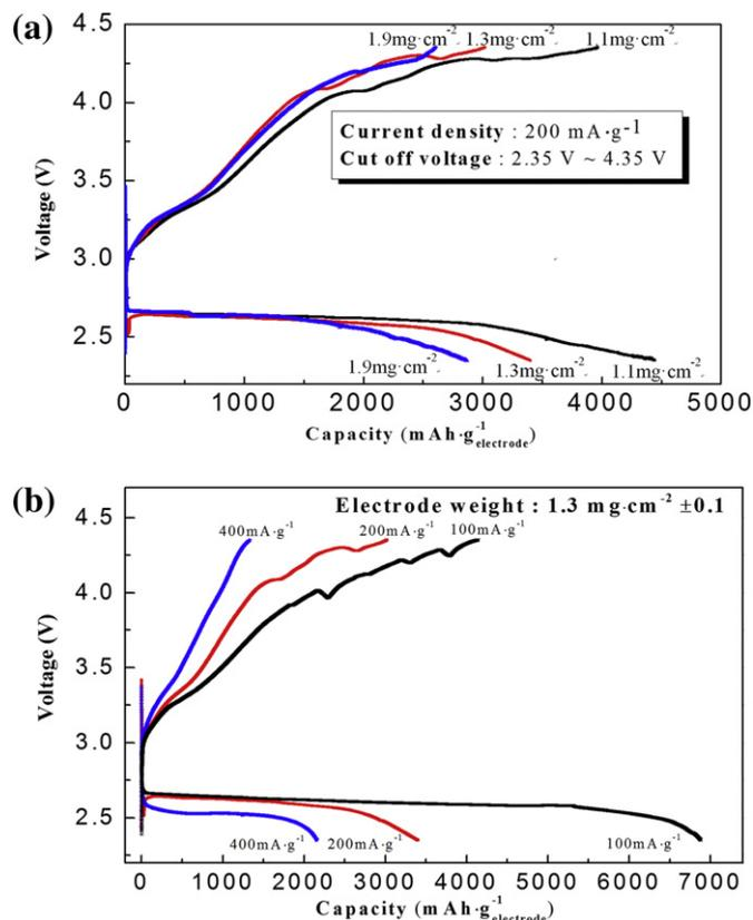
**Fig. 6.** Initial capacity of the air electrode containing carbon-sphere/ $\text{Co}_3\text{O}_4$  nanocomposite measured at a variety of (a) loading weights of electrode materials, and (b) current densities used for the test.
