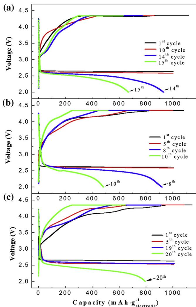
**Fig. 9.** Discharge/charge profiles of the air electrodes measured under limited capacity (1000 mAh  $g_{\text{electrode}}^{-1}$ ) and with the supply of more current at a fixed charge voltage (4.35 V): (a) electrode containing plain carbon spheres as a catalyst; (b) electrode containing commercial  $Co_3O_4$  nanopowder as a catalyst; (c) electrode containing carbon-sphere/ $Co_3O_4$  nanocomposite as a catalyst.
