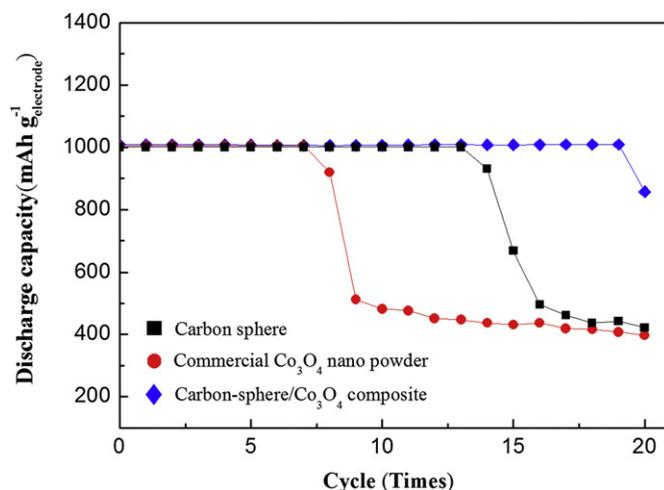
**Fig. 10.** Cyclic performance of the air electrodes measured under limited capacity (1000 mAh  $g_{\text{electrode}}^{-1}$ ) and with the supply of more current at a fixed charge voltage (4.35 V).
