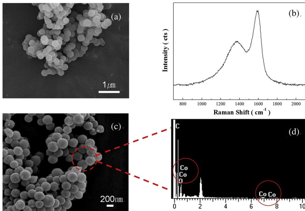
Fig. 2. (a) SEM image of the carbon sphere; (b) Raman spectroscopic profile of carbon sphere; (c) SEM image of the carbon-sphere/ $\text{Co}_3\text{O}_4$  nanocomposite; (d) SEM–EDS analysis of the surface of the composite.
