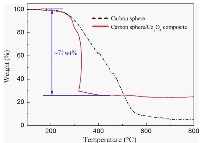
**Fig. 5.** Thermogravimetric (TG) analysis of the carbon sphere and carbon-sphere/ $\text{Co}_3\text{O}_4$  nanocomposite.
