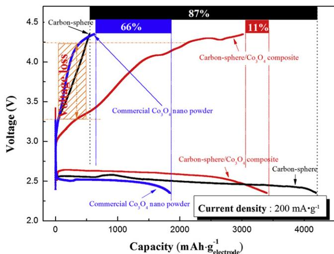
**Fig. 7.** Initial discharge/charge profiles of the air electrodes containing plain carbon spheres, commercial  $\text{Co}_3\text{O}_4$  nanopowder, and the carbon-sphere/ $\text{Co}_3\text{O}_4$  nanocomposite. The voltage range was 4.35–2.35 V and the current density was  $200 \text{ mA g}^{-1}$  (Top of the figure presents the difference between initial discharge capacity and charge capacity as %).
