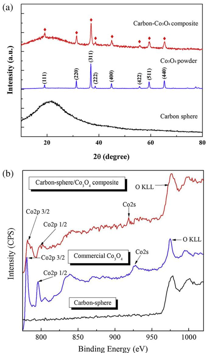
**Fig. 4.** (a) XRD patterns of carbon spheres,  $\text{Co}_3\text{O}_4$  commercial powder, and carbon-sphere/ $\text{Co}_3\text{O}_4$  nanocomposite; (b) XPS spectra of carbon spheres,  $\text{Co}_3\text{O}_4$  commercial powder, and carbon-sphere/ $\text{Co}_3\text{O}_4$  nanocomposite.
