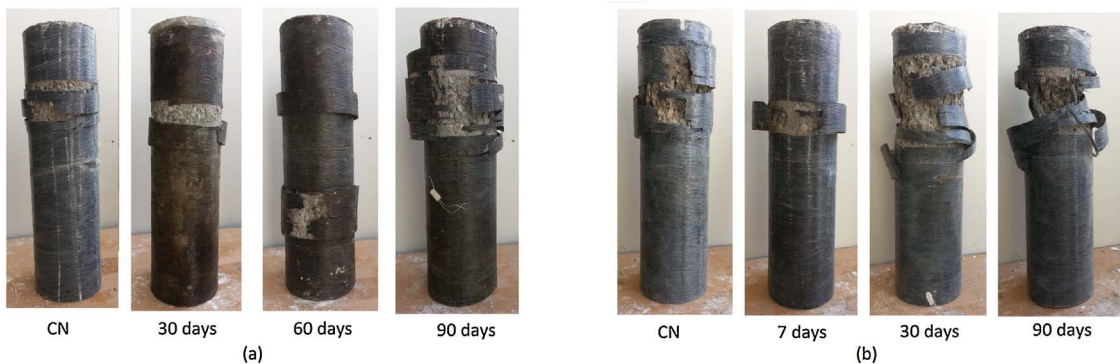
Fig. 6. Failure mode of CFRP-wrapped specimens after (a) immersion in crude oil; (b) immersion in seawater.
