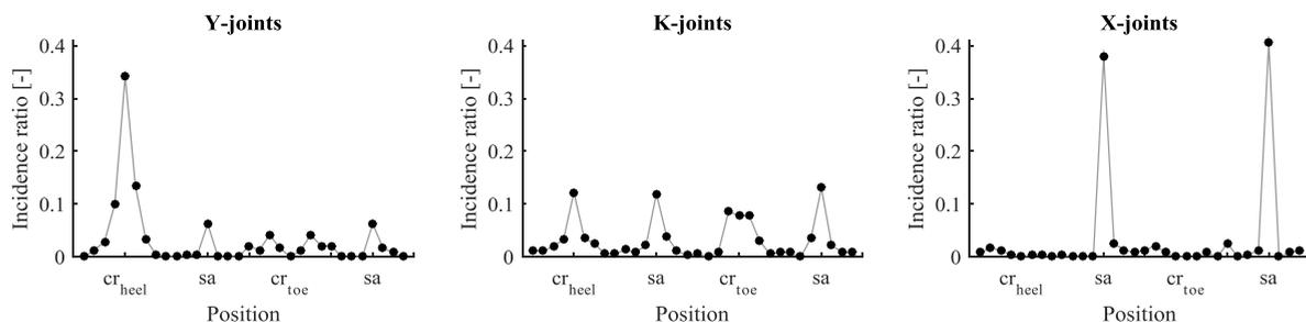
Fig. 5. Incidence ratio of highest fatigue damage per joint type plotted against the position around the circumference of the joint. Position of the crown heel (cr<sub>heel</sub>), saddles (sa), and crown toe (cr<sub>toe</sub>) are marked on the horizontal axis.
