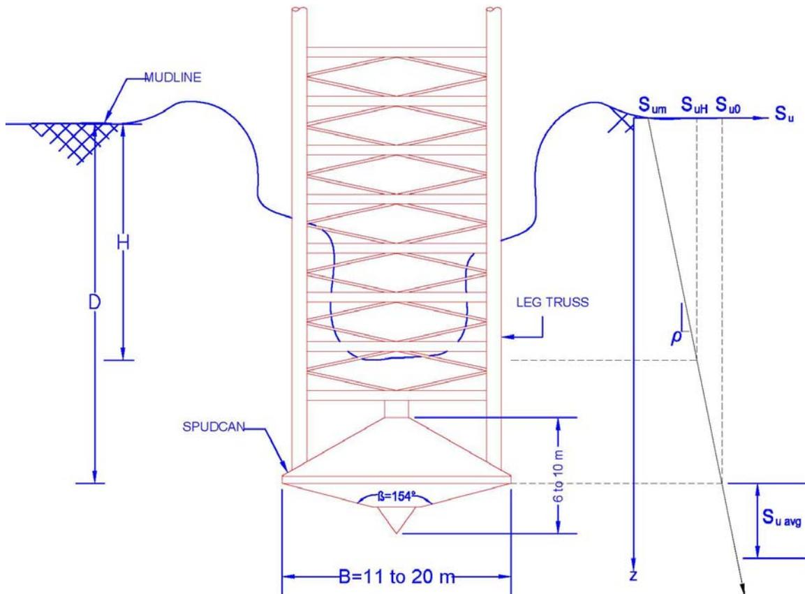
Fig. 4 Embedded Spudcan with Open Soil Cavity
