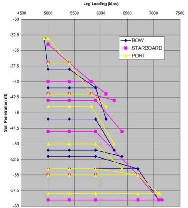
Fig. 3b Measured Spudcan Penetration Record
