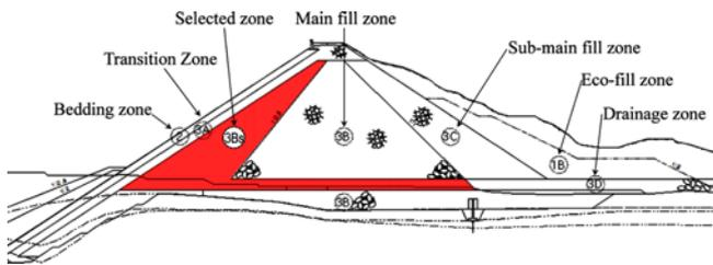
Fig. 1. Schematic Design Layout of the CFGD in This Study
