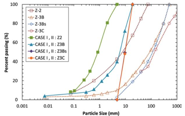
Fig. 3. Particle Size Distributions of Prototype and Model Materials
