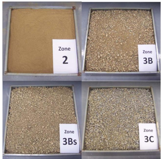
Fig. 4. Model Materials for Centrifuge Tests
