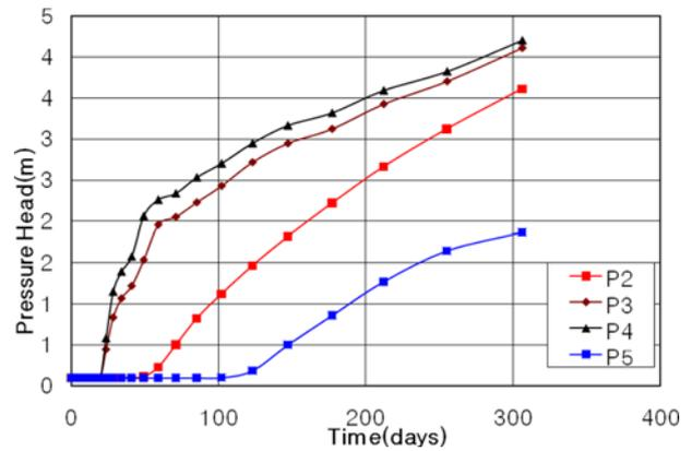
Fig. 15. Pore Water Pressure Head during Infiltration Process for CASE I with Less Permeable Zone 2 ( $k_{Zone\ 2} = 9.85 \times 10^{-8} \text{ m/s}$ )
