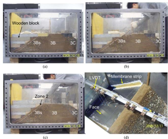
Fig. 7. Construction Procedure of Centrifuge Models: (a) Compaction of Zone 3B, (b) Compaction of Zone 3Bs, (c) Compaction of Zone 2, (d) Completion of Model Dam
