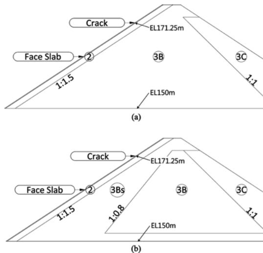
Fig. 2. Cross-sections of Centrifuge Models: (a) CASE I, (b) CASE II
