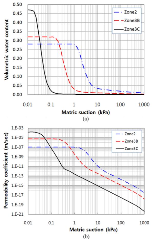
Fig. 13. Estimated Hydraulic Properties: (a) Soil-water Characteristic Curves, (b) Permeability Curves
