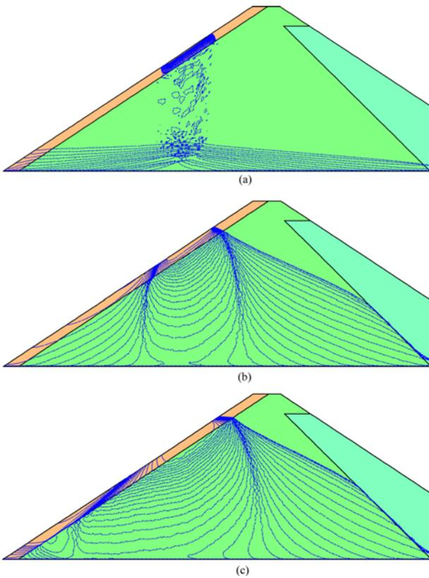
Fig. 14. Distributions of Water Front with Time during Infiltration Process for CASE I: (a)  $k_{Zone\ 2} (=9.85 \times 10^{-8} \text{ m/s}) < k_{Zone\ 3B}$ , (b)  $k_{Zone\ 2} (=5.0 \times 10^{-6} \text{ m/s}) = k_{Zone\ 3B}$ , (c)  $k_{Zone\ 2} (=5.0 \times 10^{-5} \text{ m/s}) > k_{Zone\ 3B}$
