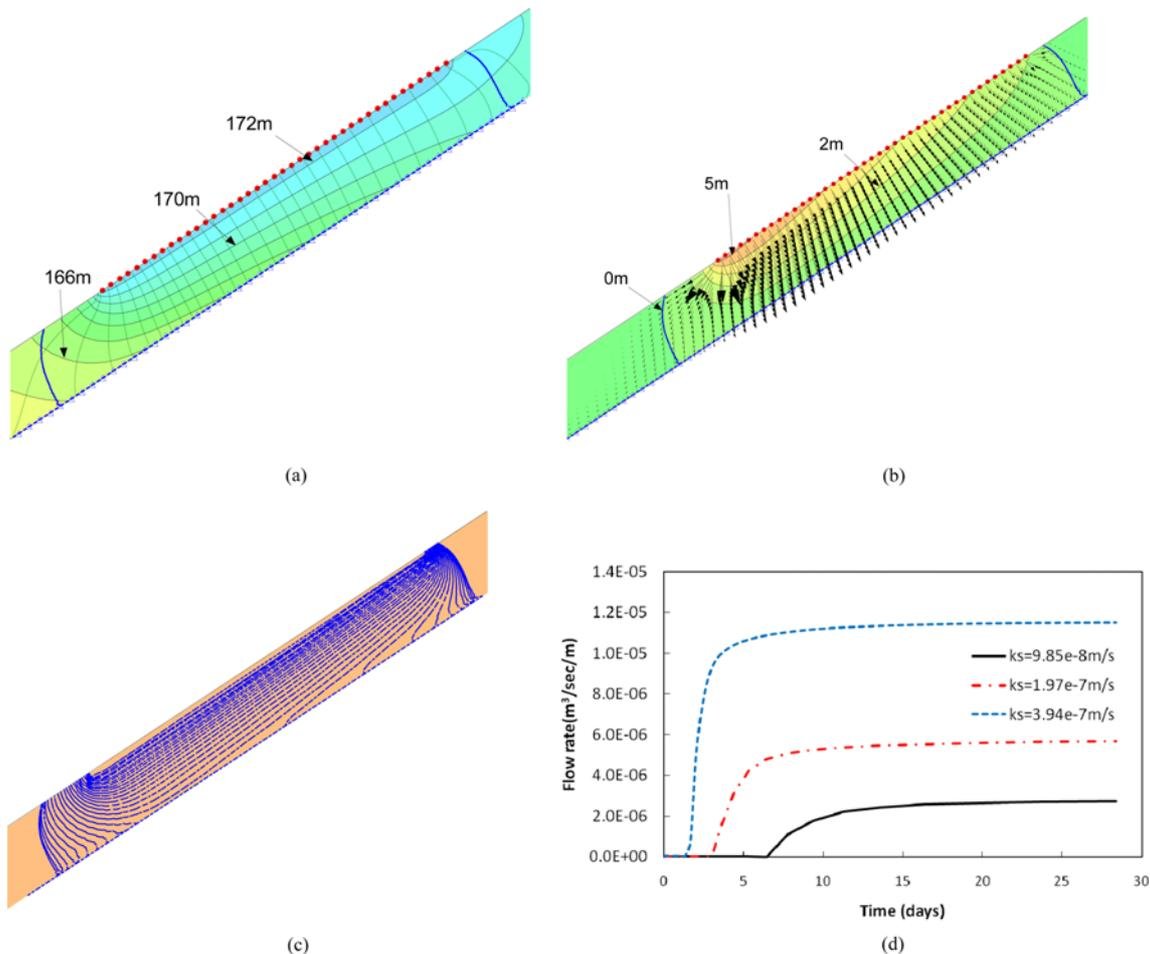
Fig. 16. Seepage Analysis Results for CASE II: (a) Total Head Contours and Flow Paths at Steady State, (b) Pore Water Pressure Head Contours and Flow Vectors at Steady State, (c) Distributions of Water Front with Time, (d) Total Outflow from Zone 2 with Time
