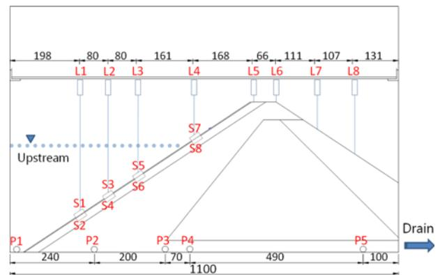
Fig. 9. Layout of Instrumented Sensors
