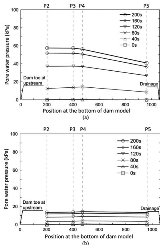
Fig. 10. Pore Water Pressure Distributions during Infiltration (In Model Time Scale): (a) CASE I, (b) CASE II
