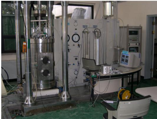
Fig. 6. Large Scale Triaxial Shear Apparatus for Permeability Tests
