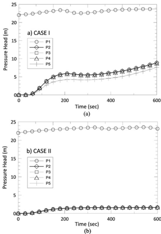
Fig. 11. Time History of Pore Water Pressure Head at Measuring Points (In Model Time Scale): (a) CASE I, (b) CASE II
