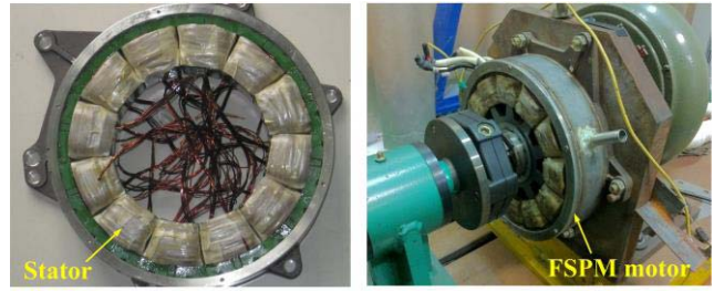
Fig. 15. Modular manufactured FSPM motor prototype.
