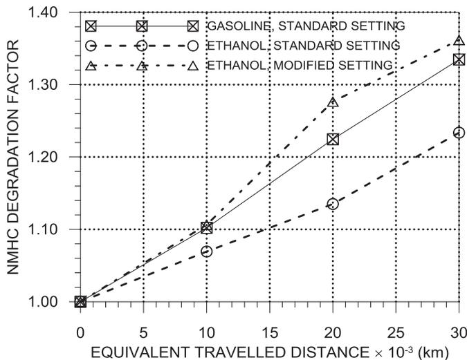
Fig. 7. Catalytic converter degradation factor for exhaust non-methane hydrocarbons conversion.
