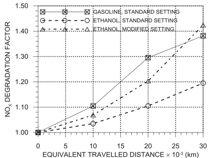
Fig. 9. Catalytic converter degradation factor for exhaust oxides of nitrogen conversion.
