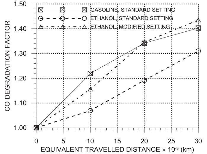
Fig. 8. Catalytic converter degradation factor for exhaust carbon monoxide conversion.
