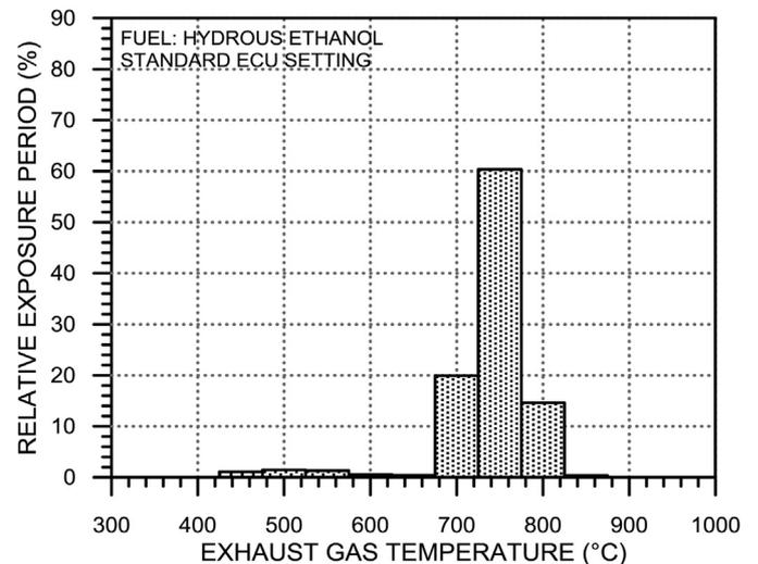
Fig. 5. Temperature histogram of the catalytic converter operating with ethanol combustion products and standard engine control setting.
