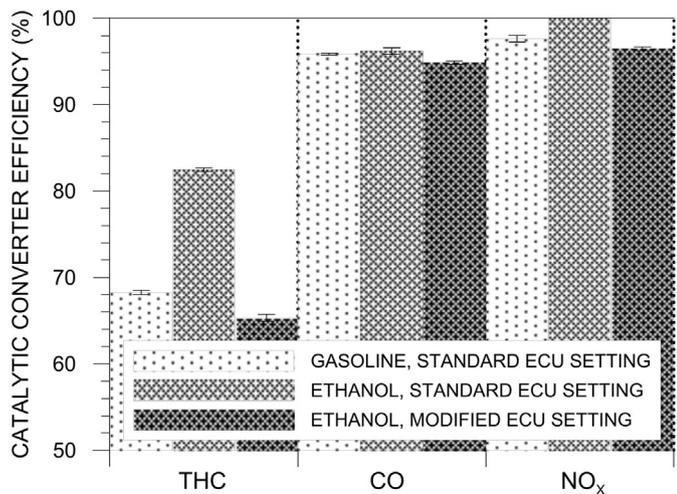
Fig. 11. Catalytic converter efficiency for conversion of synthetic gas components.
