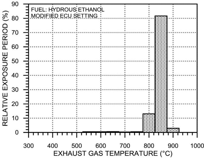
Fig. 6. Temperature histogram of the catalytic converter operating with ethanol combustion products and modified engine control setting.
