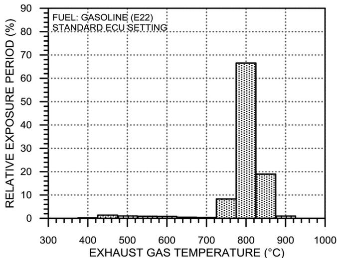
Fig. 4. Temperature histogram of the catalytic converter operating with gasoline combustion products and standard engine control setting.
