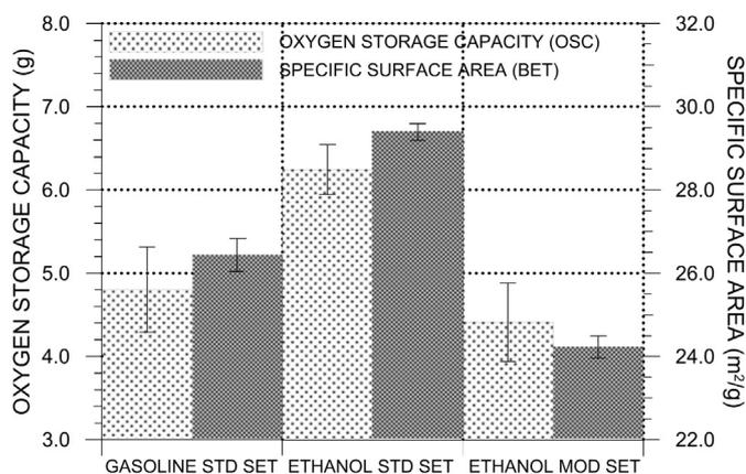
Fig. 10. Catalytic converter oxygen storage capacity (OSC) and specific surface area (BET).
