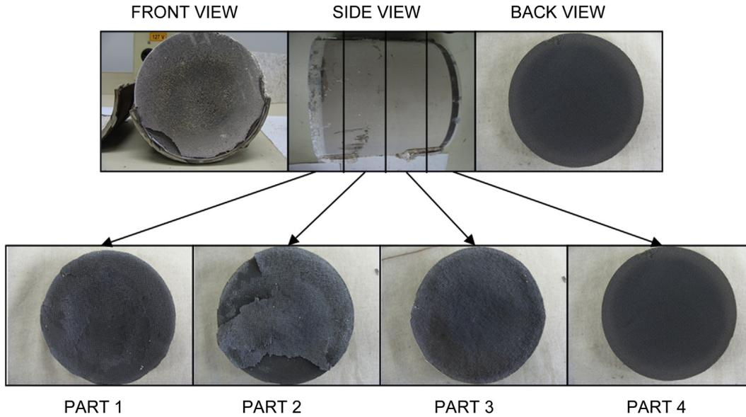
Fig. 2. Catalytic converter fractions for BET analysis.
