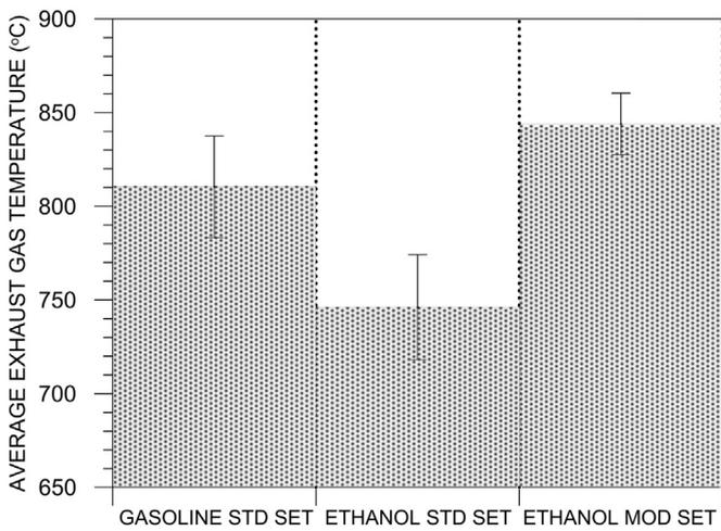
Fig. 3. Average operating temperature of the catalytic converters.
