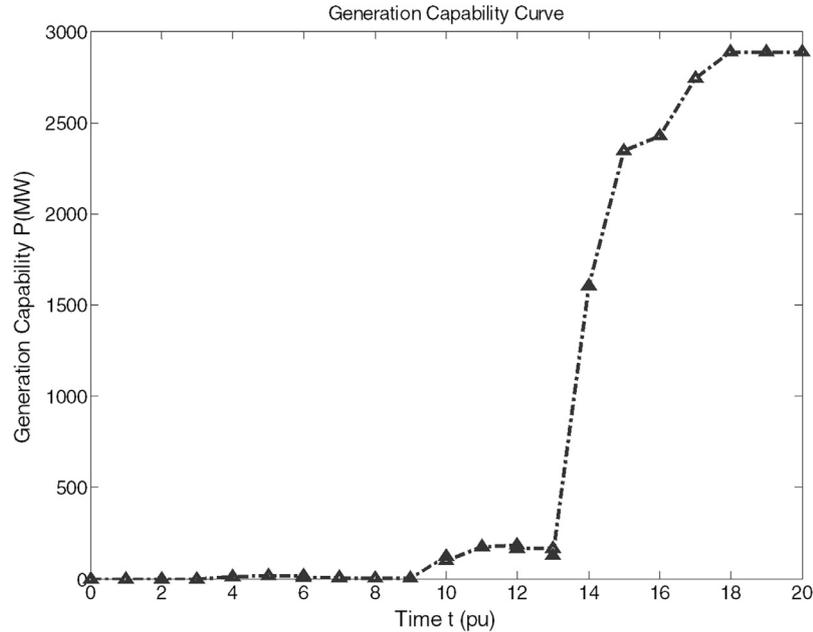
**Fig. 5.** MW generation capability curve of the ISO New England system.
