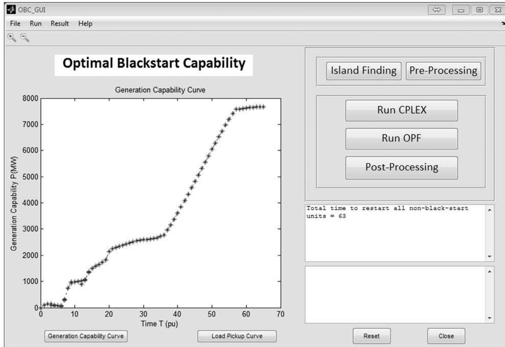
Fig. 6. MW generation capability curve of Duke Energy system.
