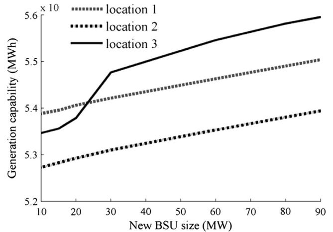
Fig. 8. MWhr generation capability curves for different BSU locations.
