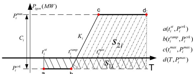
Fig. 1. Nonlinear generation capability curve.
