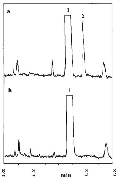
**Fig. 1** Electropherograms of fixing solution (1:25 diluted) sample before (a) and after (b) decomposition by electrolytic oxidation. Electrolyte, 50 mmol L<sup>-1</sup> borate, pH 8.5; applied voltage, 30 kV; direct UV detection at 214 nm; injection time, 4 s. Peaks: 1 - FeEDTA<sup>-</sup>; 2 - NiEDTA<sup>2-</sup>
