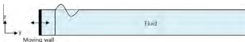
Fig. 11. Schematic of numerical model for wave generation.
